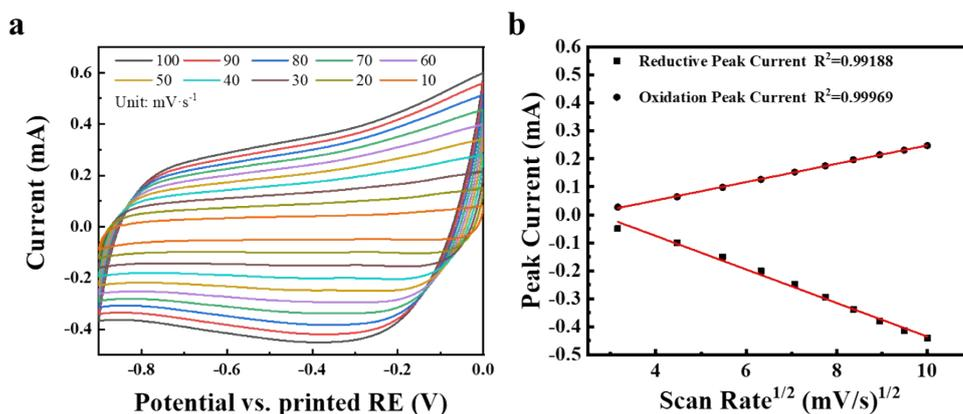
Fig. S6. (a) CV curves of printed Ag electrode modified with GA@PB at different scan rates in 10mM PBS. (b) Calibration curves of anodic and cathodic peak currents versus scanning velocity.
