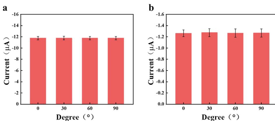
Fig. S10. The flexibility experiment about the analytical electrodes. (a) current responses of the analytical electrodes modified with GA@PB in 1 mM  $\text{H}_2\text{O}_2$ ; (b) current responses of the analytical electrodes modified with CTS/GOx-GA@PB in 300  $\mu\text{M}$  glucose.
