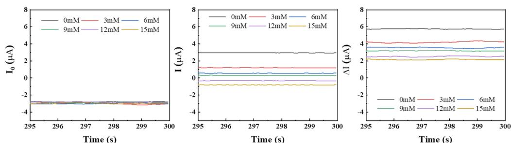
Fig. S13  $I$ ,  $I_0$  and  $\Delta I$  of the iontophoretic biosensing system on glucose sensing ranging from 0-15 mM..
