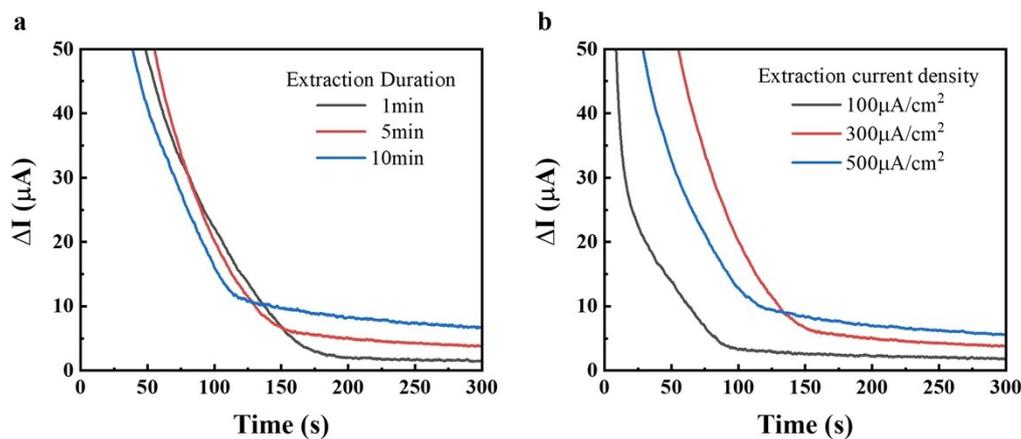
Fig. S14. Influence of extraction duration and current density during reverse iontophoresis on current responses. (A) Influence of extraction duration (extraction current density: 300  $\mu\text{A}\cdot\text{cm}^{-2}$ ). (B) Influence of extraction current density (extraction duration: 5 min).
