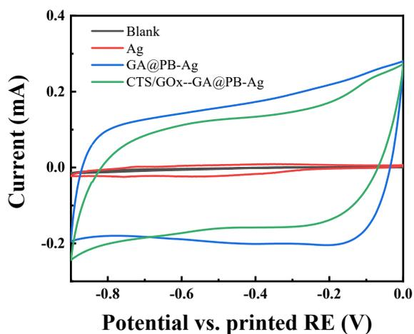
Fig. S5. CV curves of blank electrode (black line), printed Ag electrode (red line), GA@PB on Ag (denoted as GA@PB, blue line) and CTS/GOx-GA@PB on Ag (denoted as CTS/GOx-GA@PB, green line) at a scan rate of 50mV/s in 10 mM PBS.
