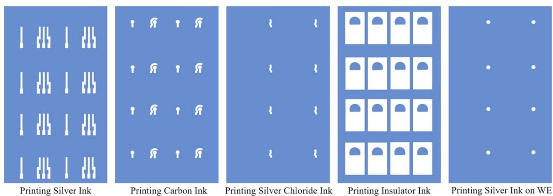
Fig. S3. Schematic diagram of the screen printing forms.
