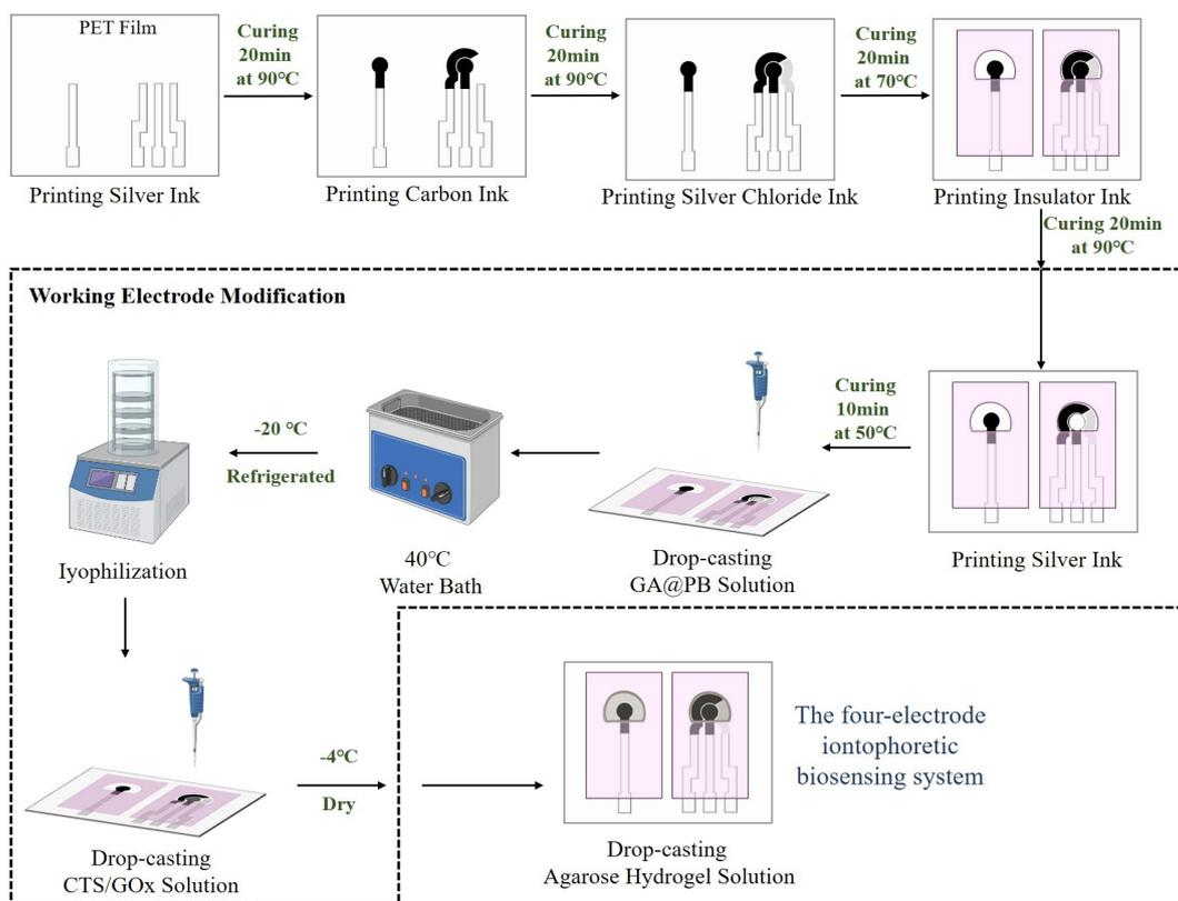
Fig. S1. Fabrication and chemical modification process of the four-electrode iontophoretic biosensing system.
