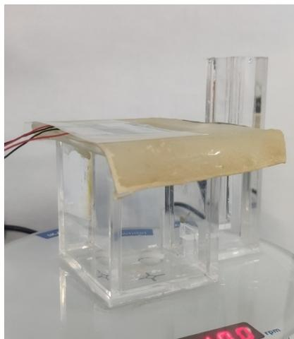
Fig. S12. Digital photograph of the self-developed reverse iontophoresis experimental platform.
