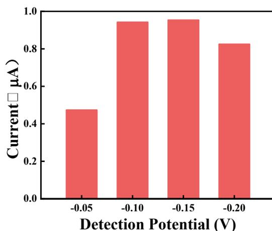
Fig. S7. Current responses of the analytical electrodes modified with CTS/GOx-GA@PB at different detection potential.
