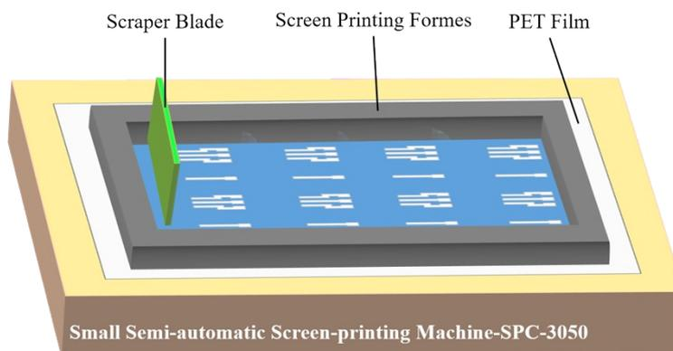
Fig. S2. Schematic diagram of screen-printing technique.
