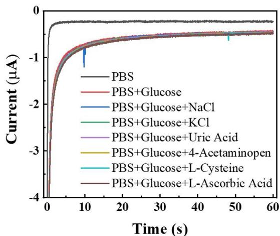
Fig. S9. Interference study. Chronoamperometric response in PBS with the presence of 50  $\mu\text{M}$  glucose and other common coexisting electroactive species.
