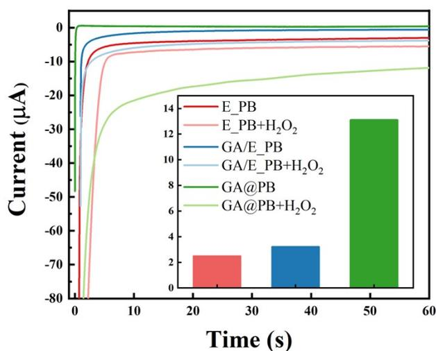
Fig. S8. Current responses of the analytical electrodes modified with electrodeposited PB (E<sub>PB</sub>, red line), GA with electrodeposited PB (GA/E<sub>PB</sub>, blue line) and GA@PB (green line) over the
