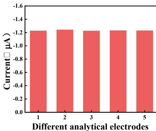
Fig. S11. Current responses of different analytical electrodes in the same glucose concentration (300  $\mu\text{M}$ ) by chronoamperometry in 10 mM PBS (pH 7.4)
