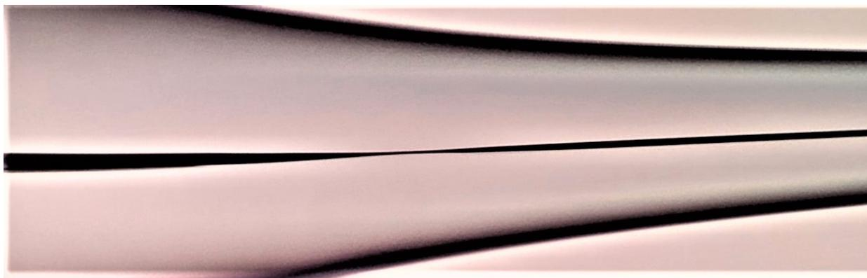
**Figure S8. Representative microscopic images of pinched Pt wire resulted from pulling.** When using a higher filament such as 4 or 5, the pinched Pt wires are observed which provide resistive and capacitive electrode.
