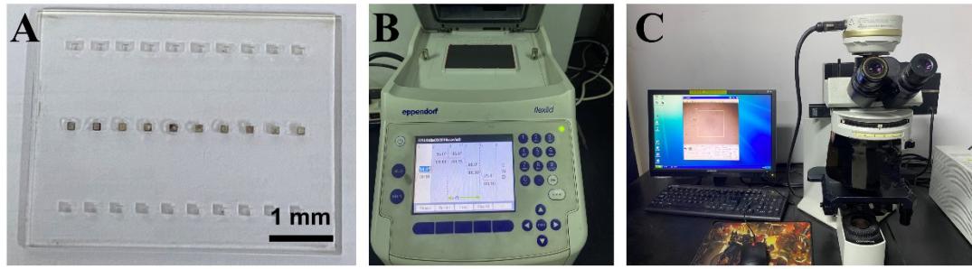
Figure S2. Physical image of the experimental setup. (A) Magnet apparatus for driving bead transfer. (B) An in-situ thermal cycler instrument used to provide the temperature cycle required for digital PCR reaction. (C) Fluorescence microscope equipped with mercury lamp and CCD image sensor for capturing fluorescence images after thermal cycling.
