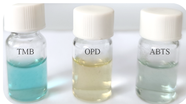
Fig. S4 The CuO/H-Gr catalyze oxidation of various peroxidase substrates in the presence of H_2O_2 to produce different color reactions.
