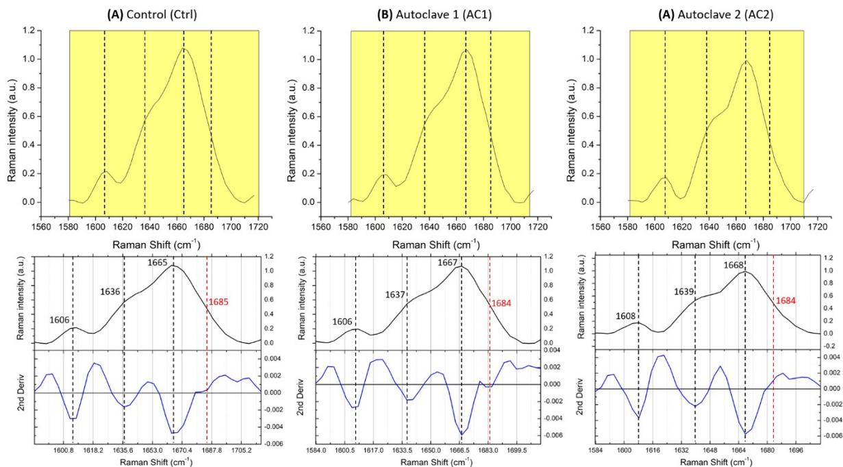
**Fig. S2. Amide I sub-peaks using 2nd derivative for SORS acquired data.** Sub-peaks identified using 2<sup>nd</sup> derivative approach for the SORS acquired data (5 mm offset is represented here) failed to identify the 4<sup>th</sup> sub-peak regardless of the sample condition i.e., control (A) or autoclaved AC1 (B) and AC2 (C).
