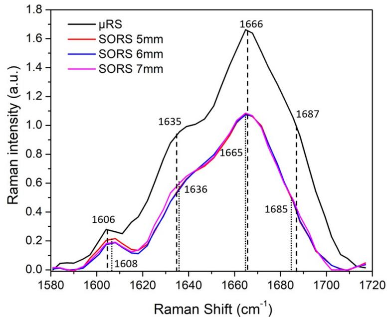
**Fig. S3. Amide I band comparison ( $\mu$ RS vs. SORS).** Raman spectra were pre-processed for background subtraction and Amide I band is separately plotted here for comparing the intensity and band shape when acquired using Raman micro-spectroscopy and SORS. Intensity of RS is higher compared to SORS irrespective of offset rings. The slight differences between peak positions are labelled. Average peak positions are used for SORS.
