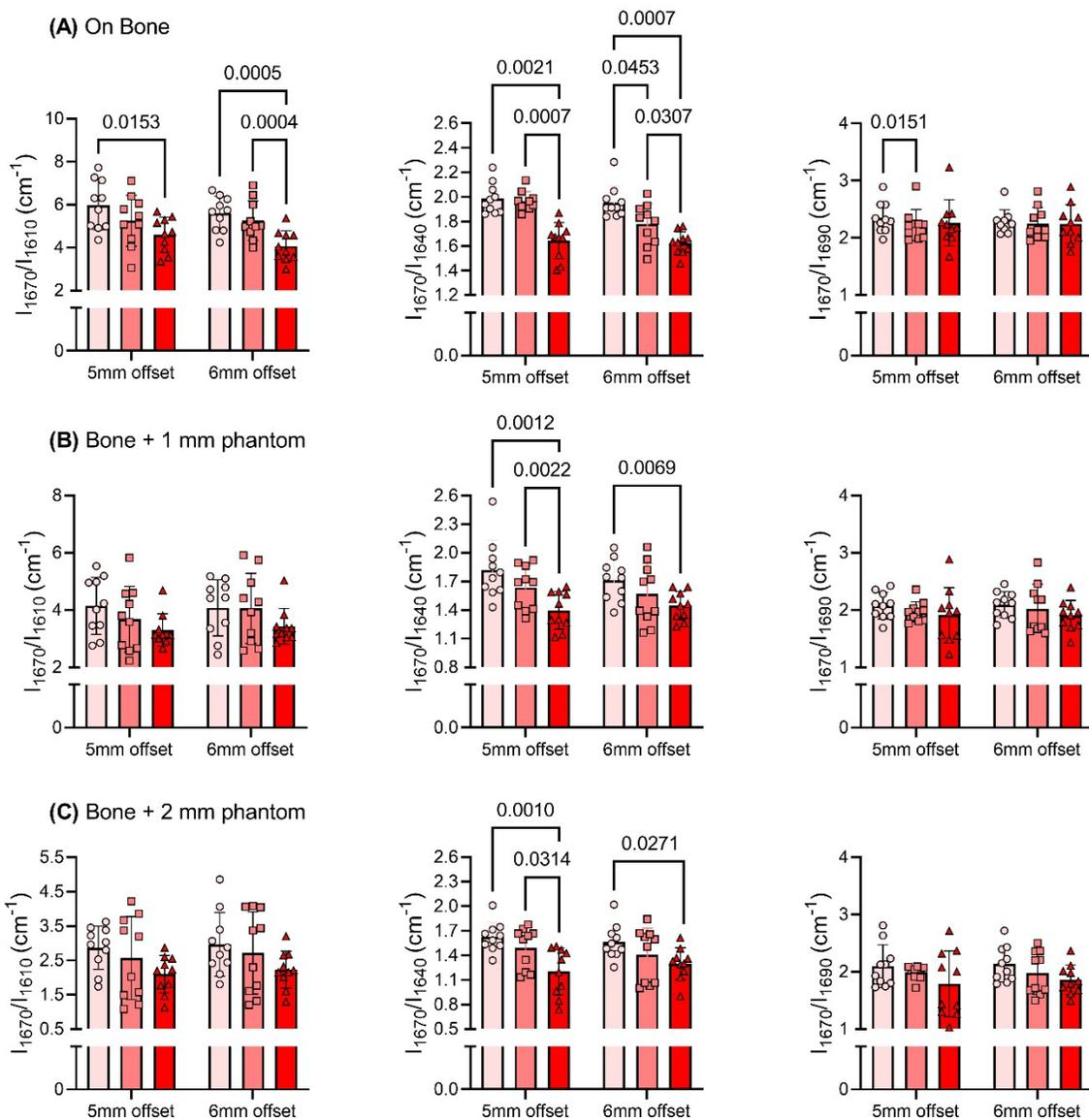
**Fig. S5. Sensitivity of SORS to autoclaving when spectra were acquired through tissue phantom layers with a thickness of 2 mm.** 4 sub-peak ratios detected through 4th derivative test are plotted against autoclave treatment for 5 mm and 6 mm offset.  $\sim I_{1670}/I_{1640}$  ratio was decreased irrespective of the layers and offsets. For other ratios ( $\sim I_{1670}/I_{1610}$ ,  $\sim I_{1670}/I_{1690}$ ) both 5 mm and 6 mm offset lost the sensitivity with layer thickness of 1 mm and 2 mm.
