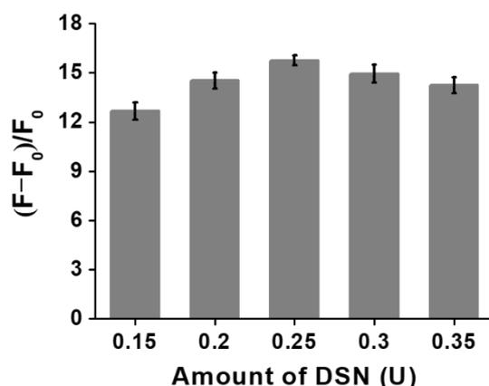
**Figure S2.** Variance of the  $(F - F_0) / F_0$  value with different amounts of DSN. The FEN1 concentration is 0.01 U/ $\mu$ L. Error bars show the standard deviation of three independent experiments.
