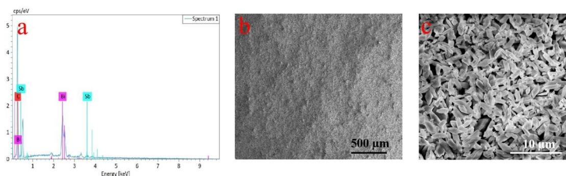
**Fig. S1.** (a) EDS of Bi-Sb AMs, (b) and (c) SEM of SPE surface modified by Bi-Sb AMs.
