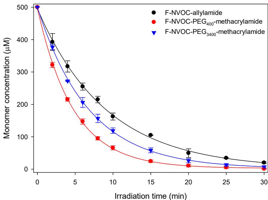
**Figure S6: Plot showing monomer concentration, determined by the peak area corresponding to M in chromatograms and molar extinction coefficient of monomer solutions, as a function of irradiation time**
