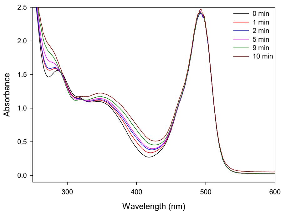
**Figure S4: UV-Vis spectra of 40 μM F-NVOC-PEG<sub>3400</sub>-methacrylamide monomer in PBS with increasing irradiation time**
