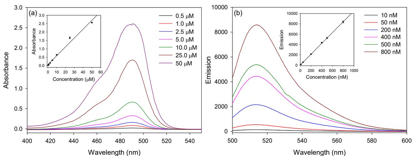
**Figure S7: (a) UV-Vis and (b) fluorescence emission spectra (excitation wavelength of 470 nm) of fluorescein in PBS where insets show peak absorbance (averaged over 485-495 nm, molar extinction coefficient at 490 nm =  $52,600 \pm 3,200 \text{ M}^{-1}\text{cm}^{-1}$ ) and emission (averaged over 509-519 nm, molar emission coefficient at 514 nm =  $(10.4 \pm 0.1) \times 10^9 \text{ M}^{-1}\text{cm}^{-1}$ ) versus fluorescein concentration**
