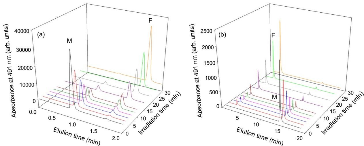
**Figure S5: HPLC waterfall plots of 1 mg/ml (a) F- NVOC-allylamide and (b) F-NVOC-PEG<sub>400</sub>-methacrylamide dissolved in acetonitrile showing increase in fluorescein (F) and decrease in photolabile monomer (M) concentrations for 0 to 30 min of irradiation time**
