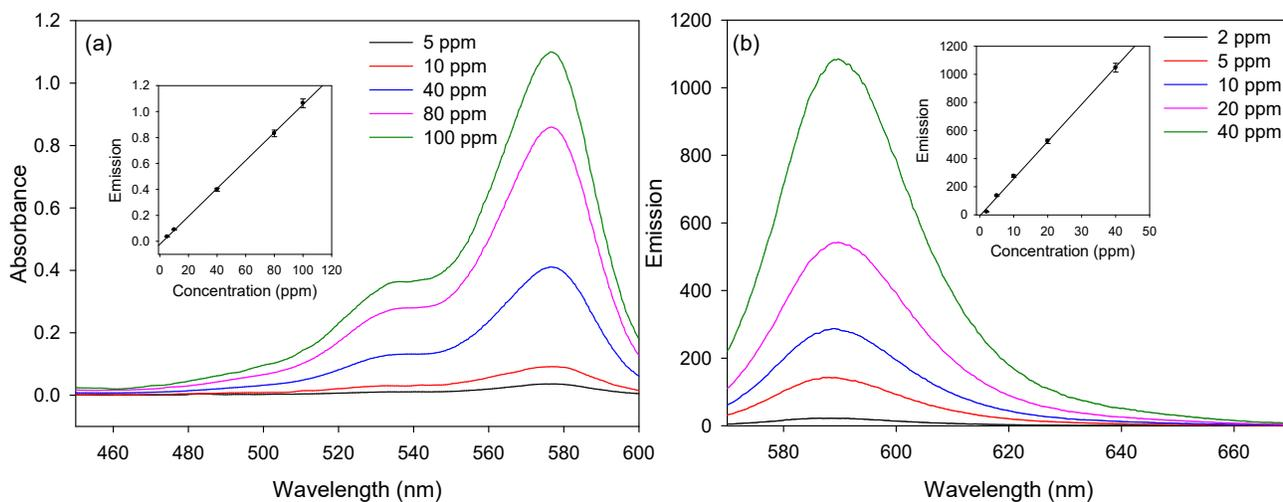
**Figure S8: (a) UV-Vis and (b) fluorescence emission spectra (excitation wavelength of 540 nm) of rhodamine-streptavidin in PBS where insets show peak absorbance (averaged over 572-582 nm, molar extinction coefficient at 577 nm =  $650,602 \pm 6,024 \text{ M}^{-1}\text{cm}^{-1}$ ) and emission (averaged over 585-595 nm, molar emission coefficient at 590 nm =  $(1.6 \pm 0.04) \times 10^9 \text{ M}^{-1}\text{cm}^{-1}$ ) versus rhodamine-streptavidin concentration**
