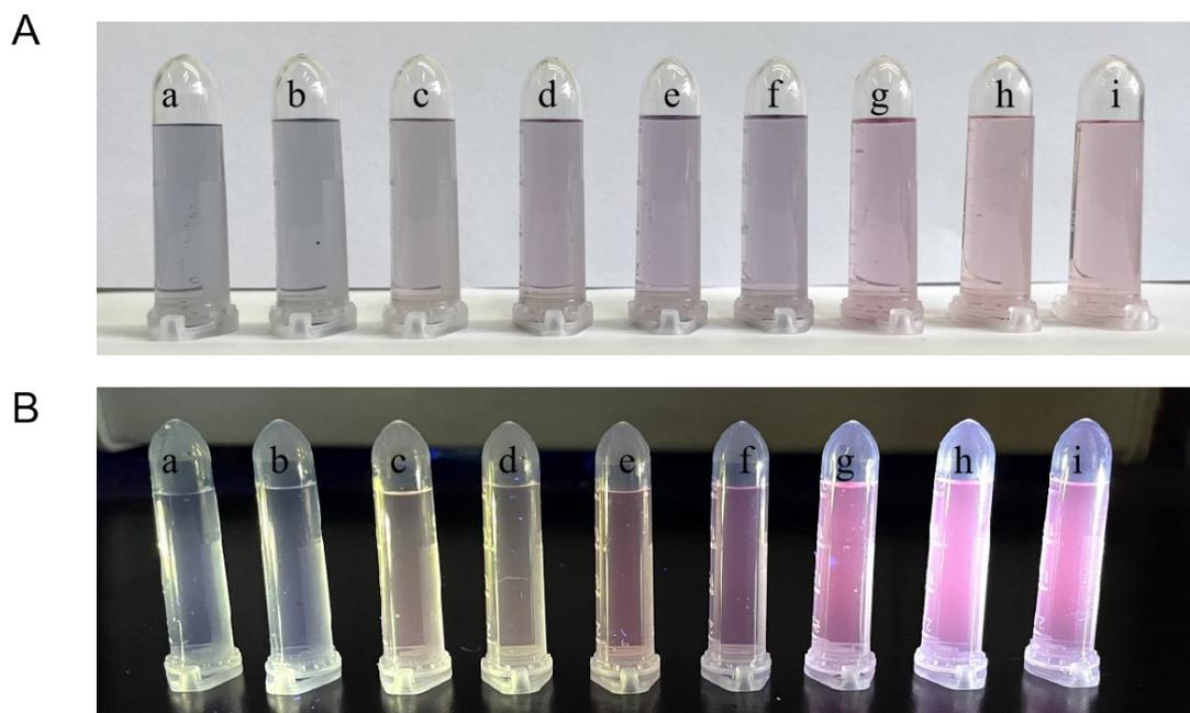
**Fig. S9.** (A) Photographs for color changes of DCO-POT chemosensory upon addition of different concentrations of ONOO<sup>-</sup> under visible light (B) Fluorescence photographs of DCO-POT (10 μM) subjected to different concentrations of ONOO<sup>-</sup> under 365nm UV light. All photos were taken by iPhone12. (From a to i: adding 0, 2, 4, 6, 8, 10, 12, 15, 20 μM ONOO<sup>-</sup>)
