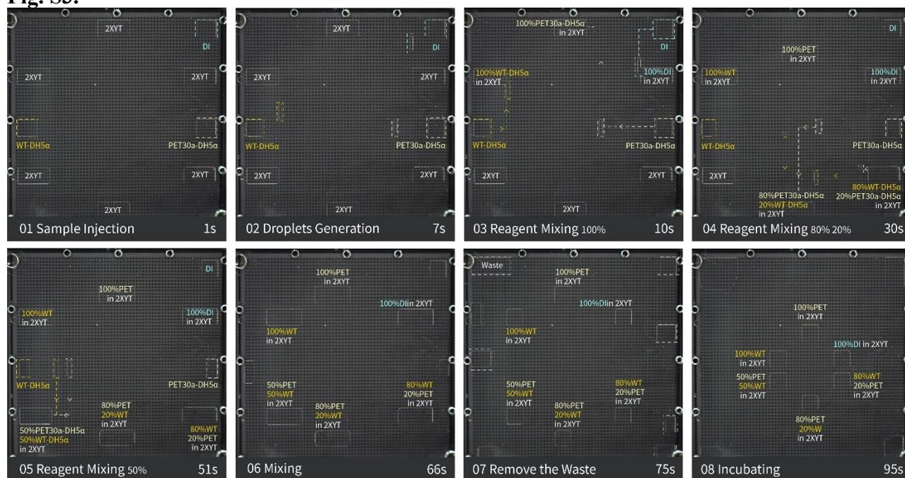
Fig S3 shows the entire process of WT-DH5 $\alpha$  and PET30a-DH5 $\alpha$  mixed and screened on a DMF chip. To prepare for the test, samples were injected into the chip's six reservoirs, and the droplets were then split, mixed and moved in a pre-programmed procedure.
