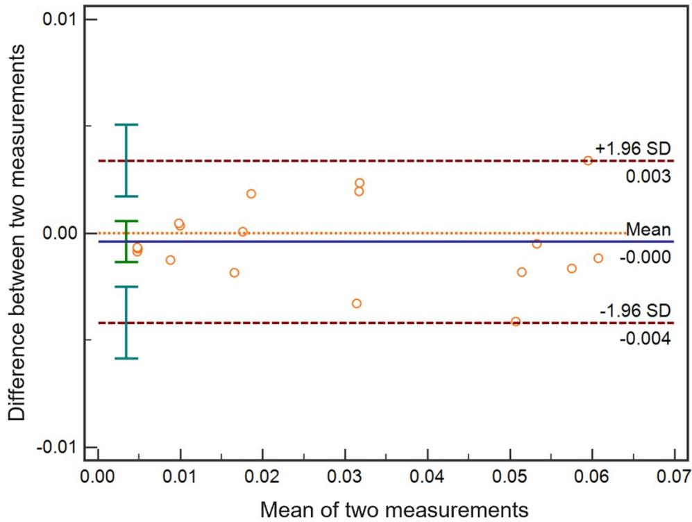
Fig S2 Bland-Altman Plot for Consistency Analysis of Protein Samples between Our System and Commercial Plate Reader
