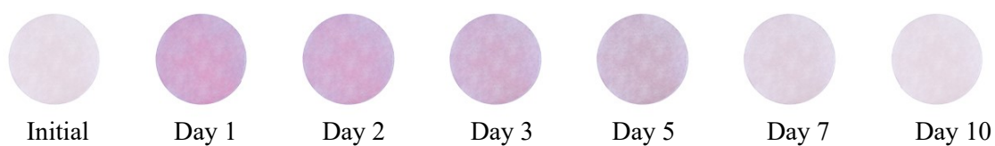
Figure 6S. Sensor image as a function of time when exposed to a constant concentration of 0.12 ppmv FA
