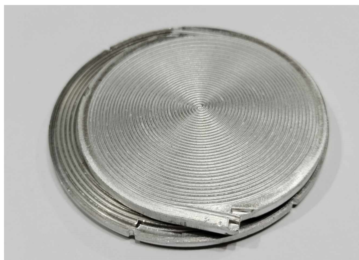
Figure S8. The size comparison between the two column disks. The disk below is a first generation column with a diameter of 8.7 cm. Another one on the top is a second generation column with a diameter of 6.2 cm, and the flow channel grooves are also smaller compared to the one below.
