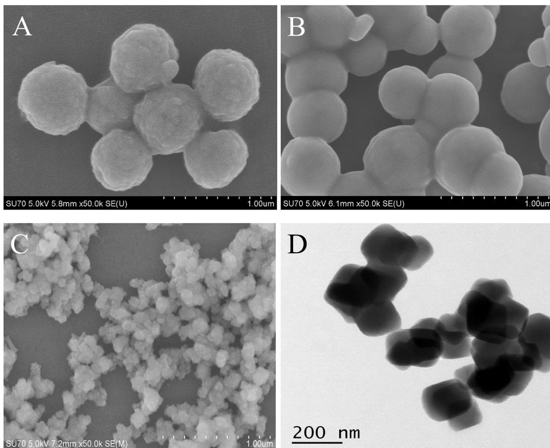
**Fig. S5** SEM of (A) mSiO<sub>2</sub> and (B) mSiO<sub>2</sub>-IgY; (C)SEM and (D) TEM of UiO-66-NH<sub>2</sub>.
