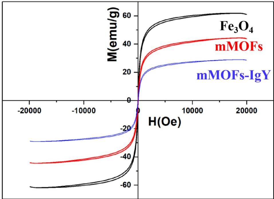
**Fig.S1** The hysteresis curve of different magnetic material.
