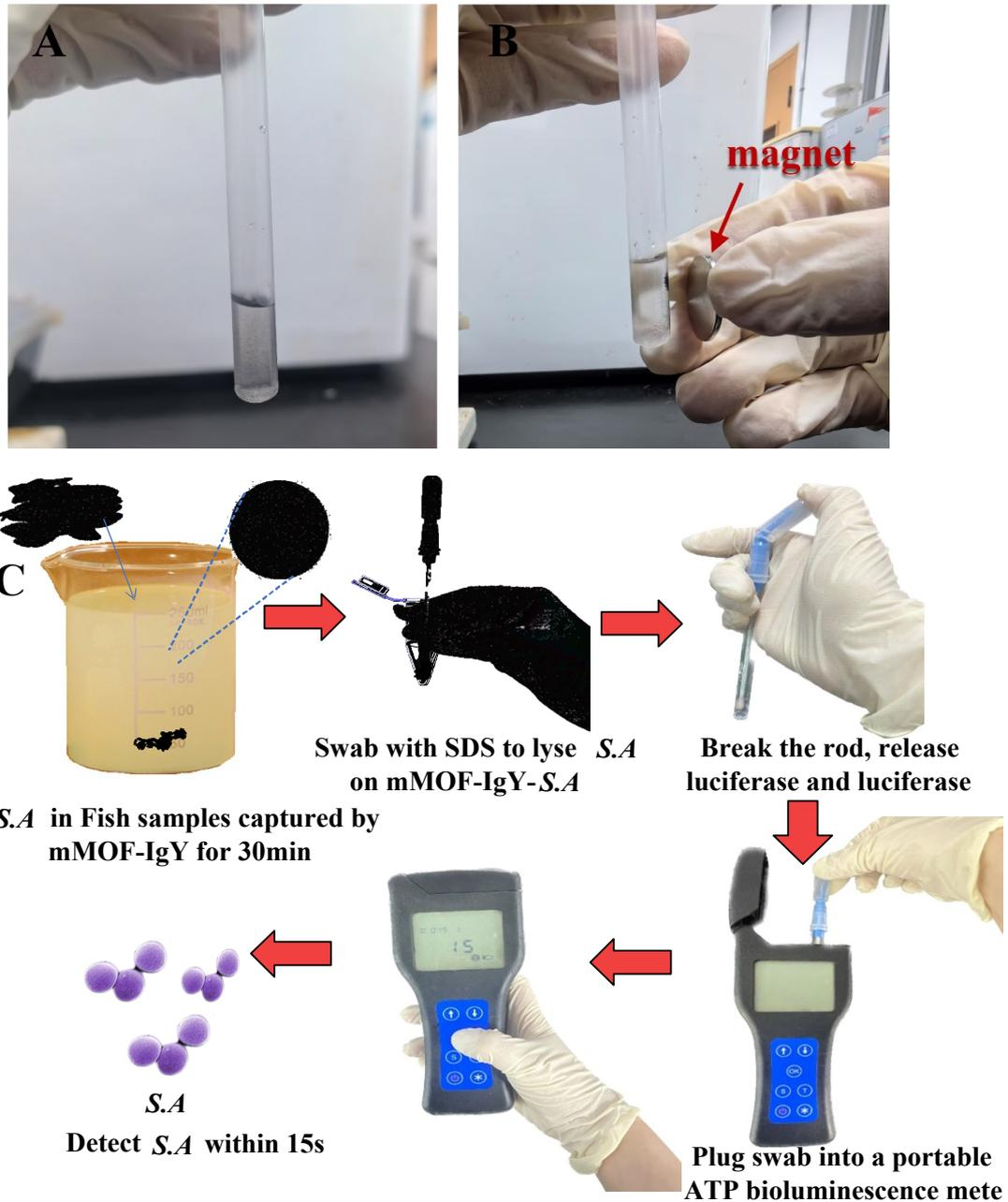
**Fig. S11** Magnetic separation process (A) before and (B) after (C) Photographs of the standard on-site detection procedures.
