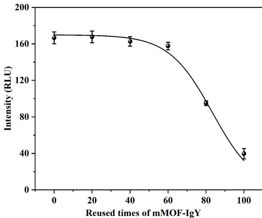
**Fig. S10** The reusability of mMOF-IgY for detection of  $10^3 \text{ CFU} \cdot \text{mL}^{-1}$  *S.A.*
