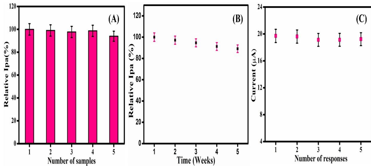
**Figure S1** (A) Reproducibility of the different CuMOF electrodes used in the detection of 0.5 mmol/L GSH in 0.1 mol/L PBS solution (pH 7.0). (B) Stability of the prepared cuMOF electrode (kept at a temperature of 4°C) used in the detection of 0.5 mmol/L GSH in PBS solution (0.1 mol/L pH 7.0) over 5 weeks. (C) Repeatability of the prepared CuMOF electrodes used in the detection of 0.5 mmol/L GSH in 0.1 mol/L PBS solution (pH 7.0).
