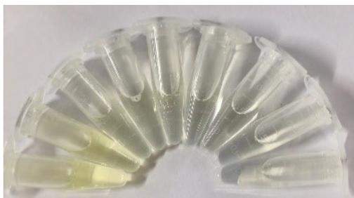
**Fig. S4** Photos of OP-CDs in different pH solutions, with pH increasing from left to right (1-9).
