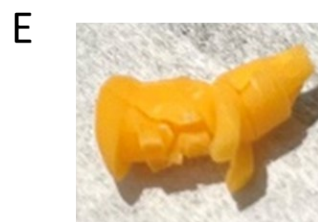
Figure S4. Compatibility between cured 3D printing resin and dimethyl sulfoxide (A&B) and ethanol (C,D,E). Raman spectra of the pure solvents are in blue and the spectrum of the solvent after an object was placed in it for 24 hours is in red. Spectra after soaking a 3D printed object for 24 hours showed a decrease in overall intensity. The object began to fall apart after soaking in DMSO for 24 hours and the solution changed to a faint orange color as shown in photograph B. Photograph D shows the object still intact while in solution, but after the object was removed and dried, it began to crack.
