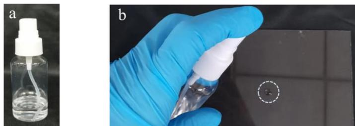
**Figure S8.** (a) A spray bottle loaded with 0.2 mM PCS and 1.6 mM KOH ethanol solution. (b) Spraying the ethanol solution of PCS and KOH to CEES contaminated surface.
