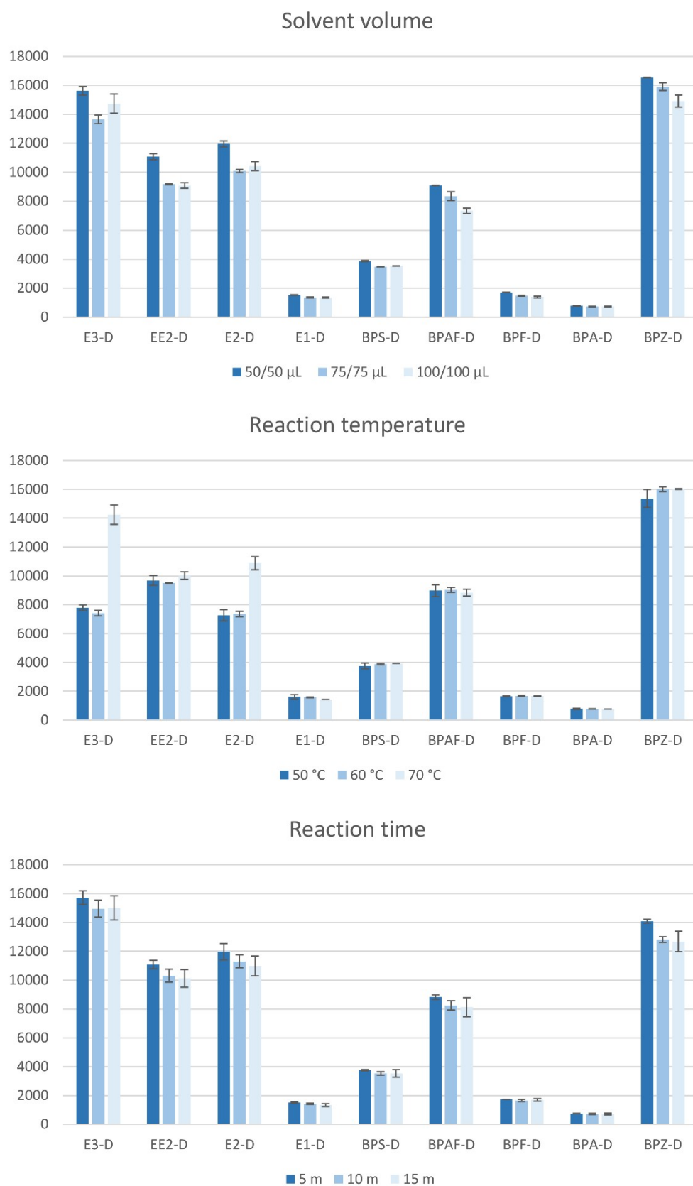
Fig. S3 Signal intensity comparison expressed as slopes of calibration curves of derivatized analytes (with standard deviation error bars) in relation to variations in derivatization parameters
