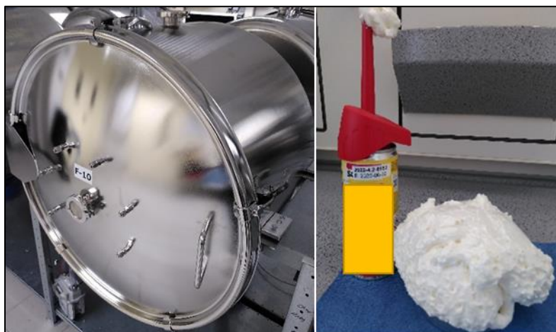
Figure S2: Emission test chamber and commercial polyurethane foam sealant considered in the emission test
