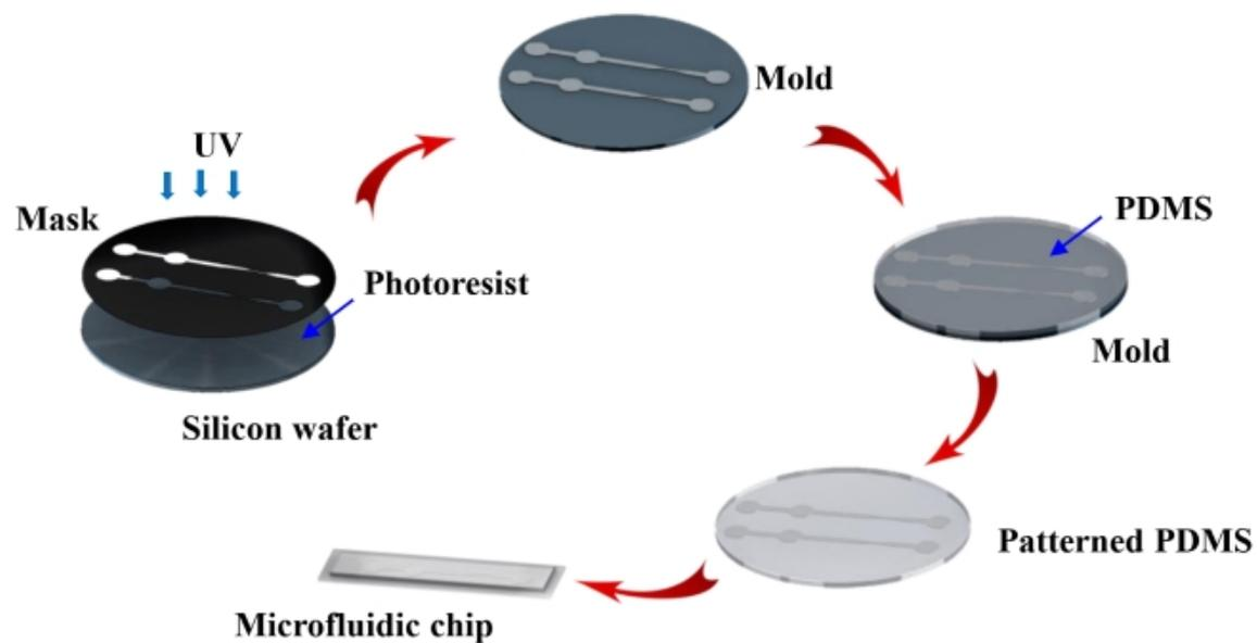
**Scheme S1** The process of making the microfluidic chip.
