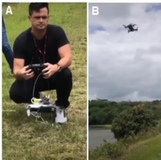
Figure S4. (A) Image of the lab-on-a-drone before the flight with the operator in control. (B) Lab-on-a-Drone flying over the region to collect water samples.
