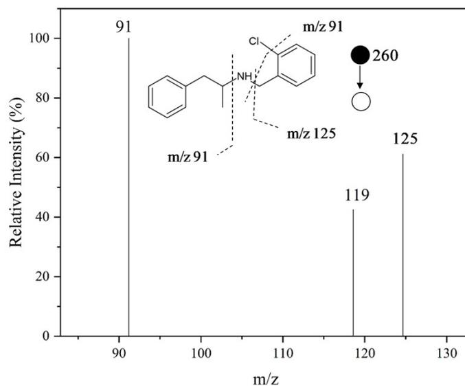
**Fig. 4S** PS(+)-MS/MS of clobenzorex. Conditions: support, blotter paper; spray solvent, MeOH:ACN (1:1 v/v); spray solvent volume, 10  $\mu$ L; spray voltage, 4.5 kV; distance between paper tip and MS inlet, 10 mm; energy collision, 5 V.
