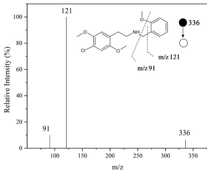
**Fig. 8S** PS(+)-MS/MS of 25C-NBOMe. Conditions: support, filter paper; spray solvent, MeOH; spray solvent volume, 10  $\mu$ L; spray voltage, 4.5 kV; distance between paper tip and MS inlet, 10 mm; energy collision, 5 V.
