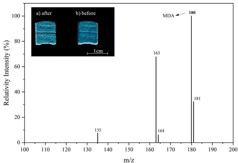
**Fig. 11S** PS(+)-MS spectrum of MDA after the 10 consecutive extractions with blotter paper and methanol as spray solvent. Photos of sample after 1 extraction and 10 consecutive extractions.
