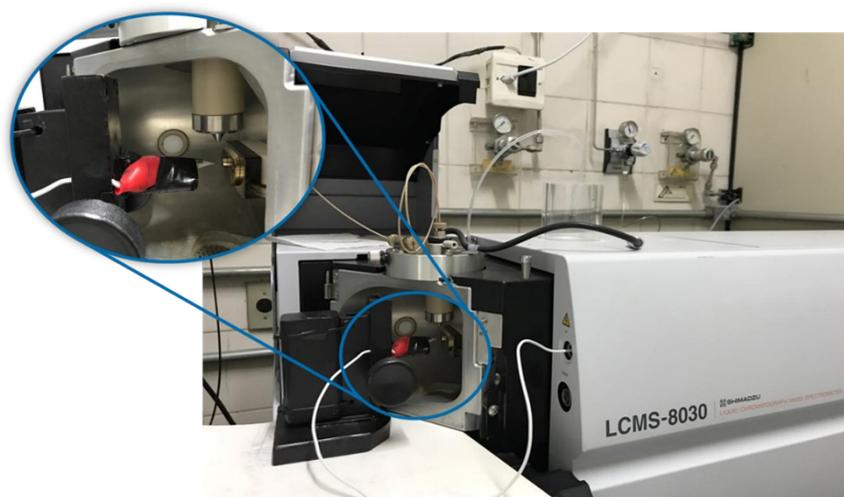
**Fig. 1S** Picture of the PS interface adapted on a Shimadzu mass spectrometer model LCMS 8030.
