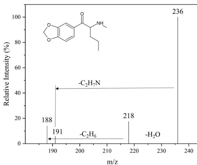
**Fig. 3S** PS(+)-MS/MS of pentylone recorded from a sample also containing NEP. Conditions: support, filter paper; spray solvent, MeOH; spray solvent volume, 10  $\mu$ L; spray voltage, 4.5 kV; distance between paper tip and MS inlet, 10 mm; energy collision 5 V.
