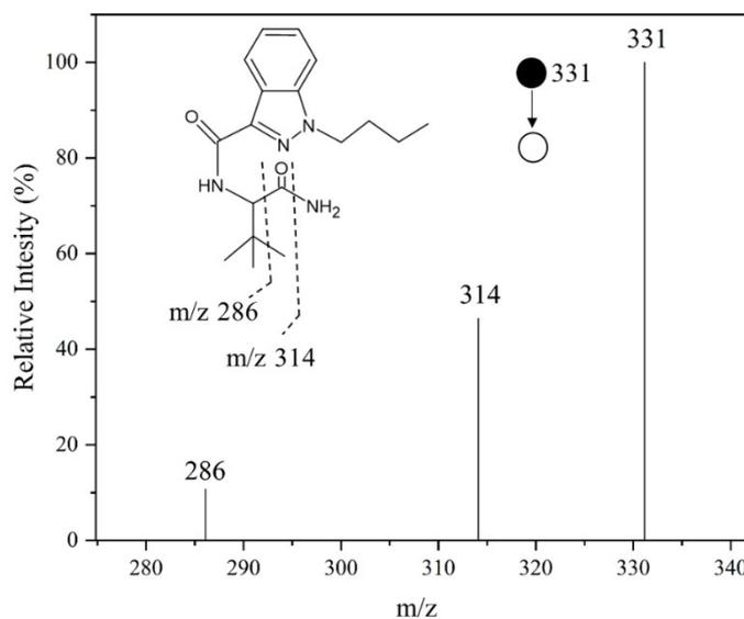
**Fig. 7S** PS(+)-MS/MS of ADB-BUTINACA. Conditions: support, filter paper; spray solvent, MeOH; spray solvent volume, 10  $\mu$ L; spray voltage, 4.5 kV; distance between paper tip and MS inlet, 10 mm; energy collision, 5 V.
