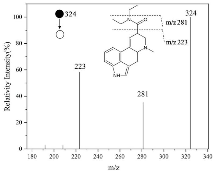
**Fig. 10S** PS(+)-MS/MS of 25C-NBOMe. Conditions: support, filter paper; spray solvent, MeOH; spray solvent volume, 10  $\mu$ L; spray voltage, 4.5 kV; distance between paper tip and MS inlet, 10 mm; energy collision, 20 V.
