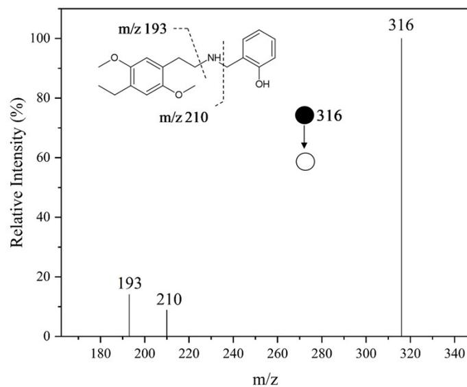
**Fig. 9S** PS(+)-MS/MS of 25E-NBOH. Conditions: support, blotter paper; spray solvent, MeOH:ACN (1:1 v/v); spray solvent volume, 10  $\mu$ L; spray voltage, 4.5 kV; distance between paper tip and MS inlet, 10 mm; energy collision, 5 V.
