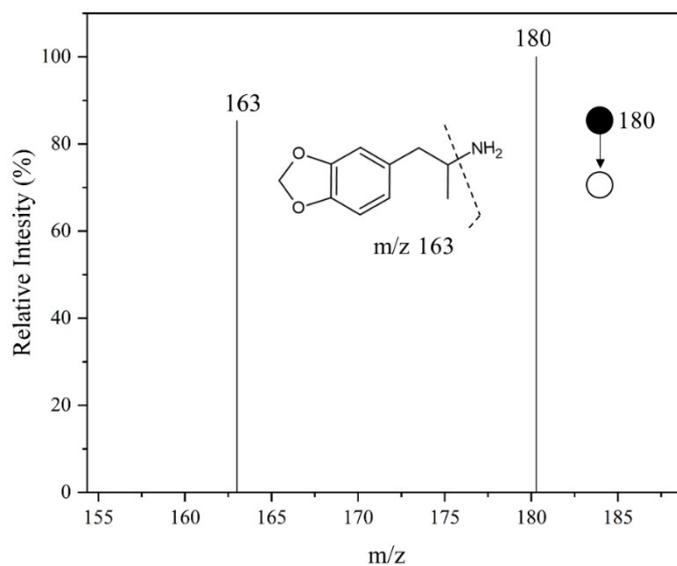
**Fig. 5S** PS(+)-MS/MS of MDA. Conditions: support, blotter paper; spray solvent, MeOH; spray solvent volume, 10  $\mu$ L; spray voltage, 4.5 kV; distance between paper tip and MS inlet, 10 mm; energy collision, 5 V.
