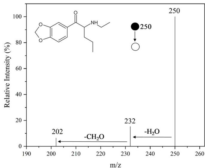
**Fig. 2S** PS(+)-MS/MS of *N*-ethylpentylone (NEP) recorded from a sample also containing U-47700 (a potent synthetic opioid also known as pink heroin). Conditions: support, filter paper; spray solvent, MeOH; spray solvent volume, 10  $\mu$ L; spray voltage, 4.5 kV; distance between paper tip and MS inlet, 10 mm; energy collision 5 V.
