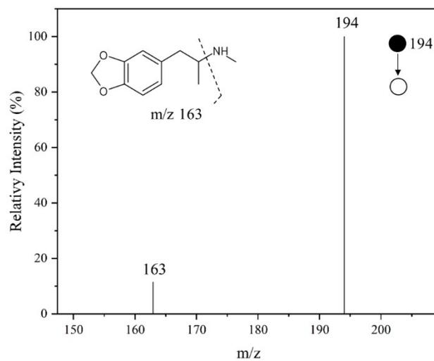
**Fig. 6S** PS(+)-MS/MS of MDMA. Conditions: support, blotter paper; spray solvent, MeOH; spray solvent volume, 10  $\mu$ L; spray voltage, 4.5 kV; distance between paper tip and MS inlet, 10 mm; energy collision, 5 V.
