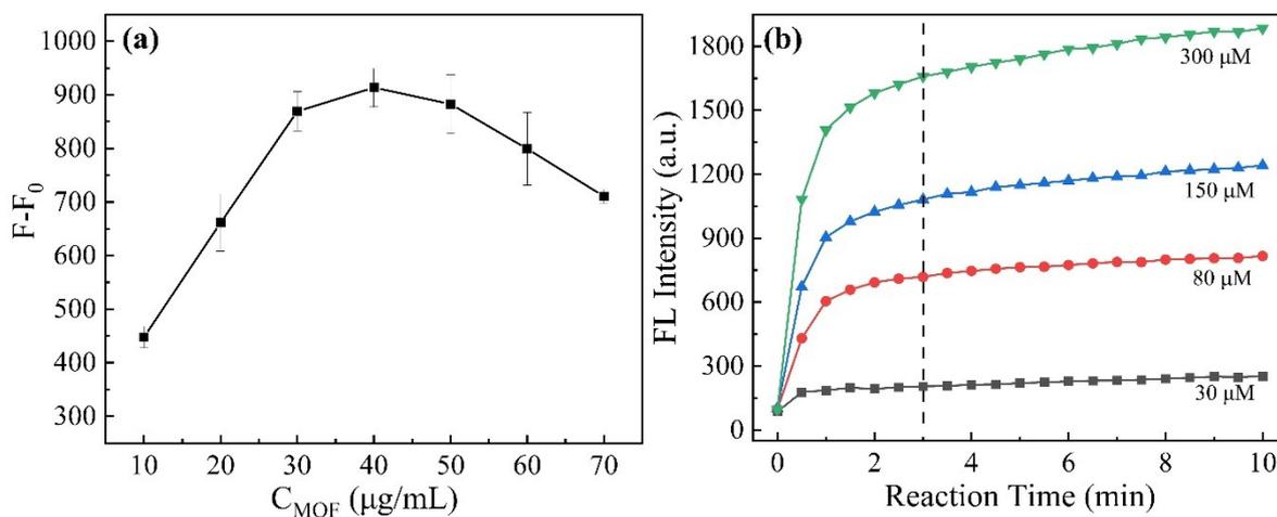
Fig. S5. Optimization of the conditions for UiO-66-NH<sub>2</sub> detection of DCP concentration in aqueous solution (a) UiO-66-NH<sub>2</sub> concentration, (b) Reaction time.
