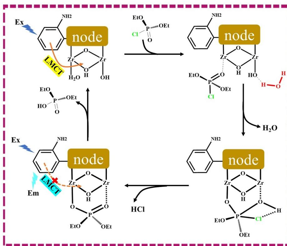
Fig. S3. The reaction process of UiO-66-NH<sub>2</sub> with DCP and the mechanism of LMCT process change.
