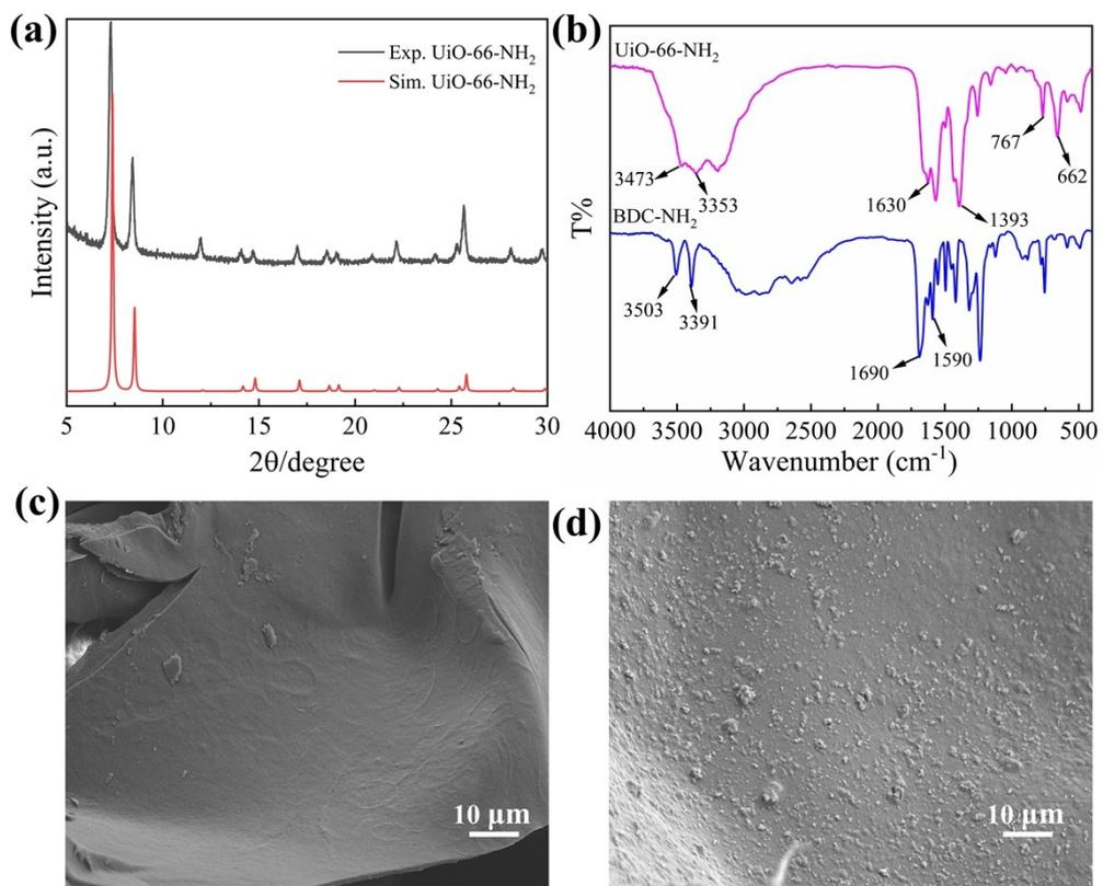
Fig. S1. (a) PXRD patterns of UiO-66-NH<sub>2</sub> and simulated UiO-66-NH<sub>2</sub>, (b) FT-IR plots of UiO-66-NH<sub>2</sub> and BDC-NH<sub>2</sub>, (c) SEM image of Aga hydrogel, (d) SEM image of UiO-66-NH<sub>2</sub>@Aga.
