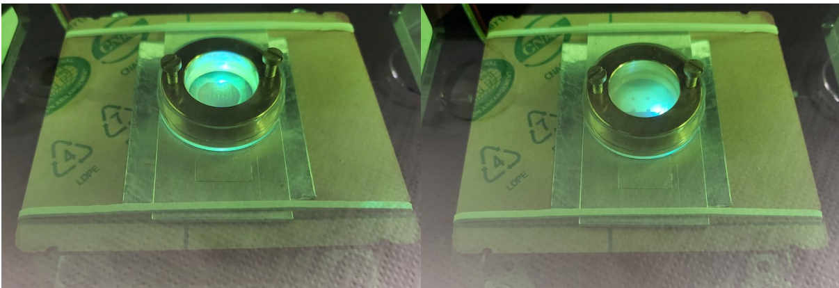
Figure S2. SERS substrate preparation. The AgNWs layer on the PTFE membrane is processed with the engraver machine in ethanol solution to remove selected areas of the silver surface and obtain 4 spots of 1 mm of diameter: (A) initial AgNWs layer engraving and (B) final AgNWs layer engraving process.
