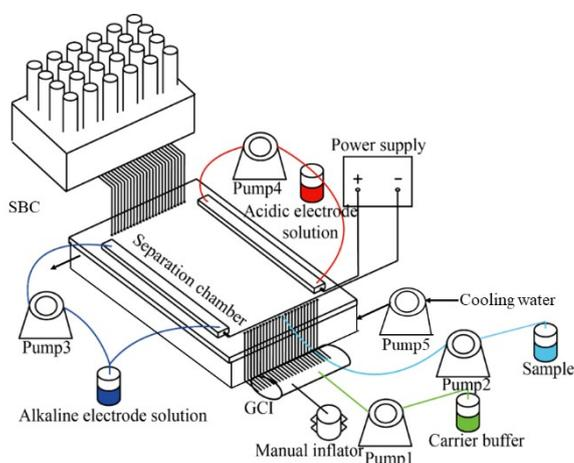
**Figure S1.** Schematic of the overall free-flow electrophoresis unit. Including gas-liquid buffer (GCI), separation chamber, cooling device, self-balancing collection device (SBC), power supply, and pump system consisting of buffer solution drive pump (Pump 1), sample pump (Pump 2), electrode buffer circulation pump (Pump 3,4), and cooling water circulation pump (Pump 5).
