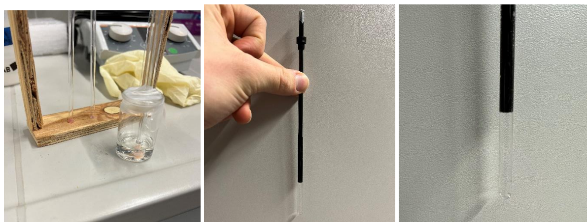
Figure S20. Images of alternative NMR tube setups including a pig intestine as alternative barrier (left) as well as 3D-printed inserts (mid and right) to substitute the glass tubes.
