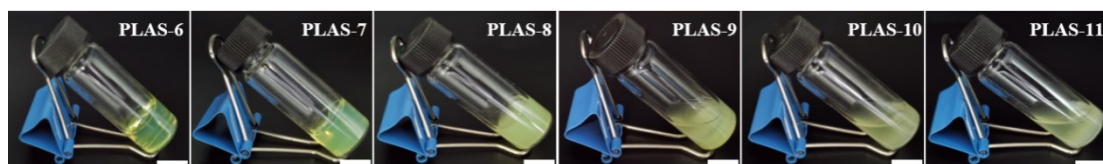
Fig. S5 Photographs of gelation behaviors of PLAS with different monomer concentrations.
