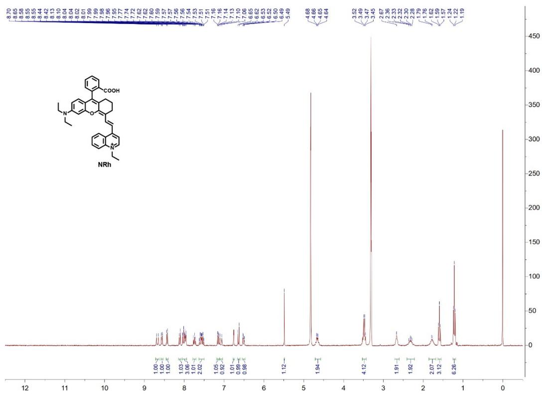
Fig. S1 The  $^1\text{H}$  NMR spectrum of compound NRh.
