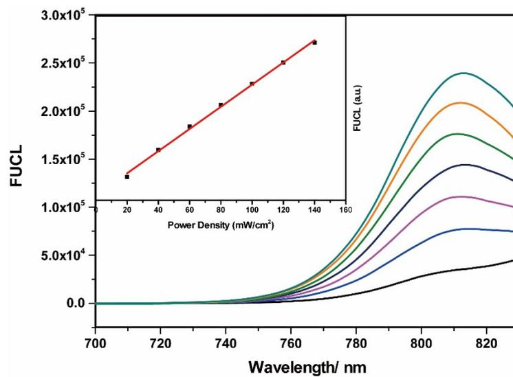
**Fig. S6** FUCL emission spectra of NRh in ethanol at different power density. (Insert: FUCL emission intensity as a function of power density (Ex = 850 nm).
