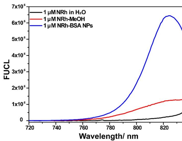
**Fig. S9** FUCL emission spectra of NRh, NRh-BSA NPs in H<sub>2</sub>O and NRh in MeOH.
