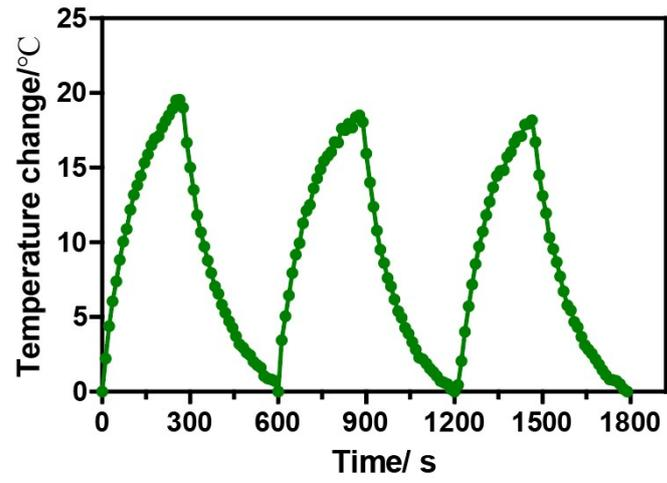
**Fig. S11** Heating and cooling curves of NRh-BSA NPs for three cycles by turning on and off laser.
