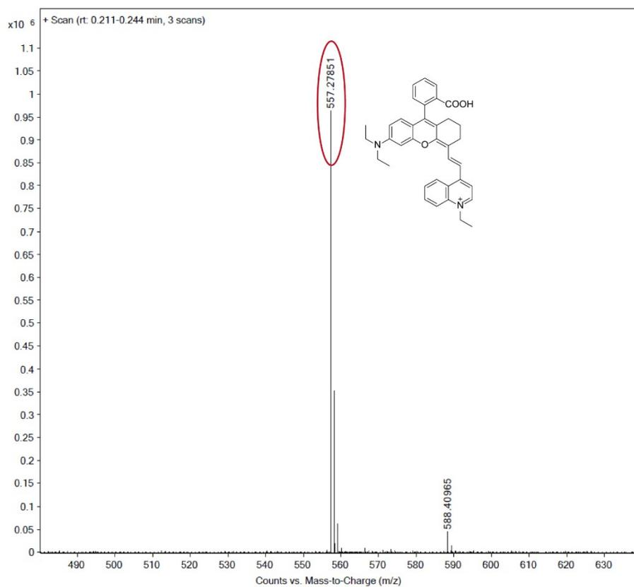
**Fig. S3** High-resolution mass spectra of compound **NRh**.
