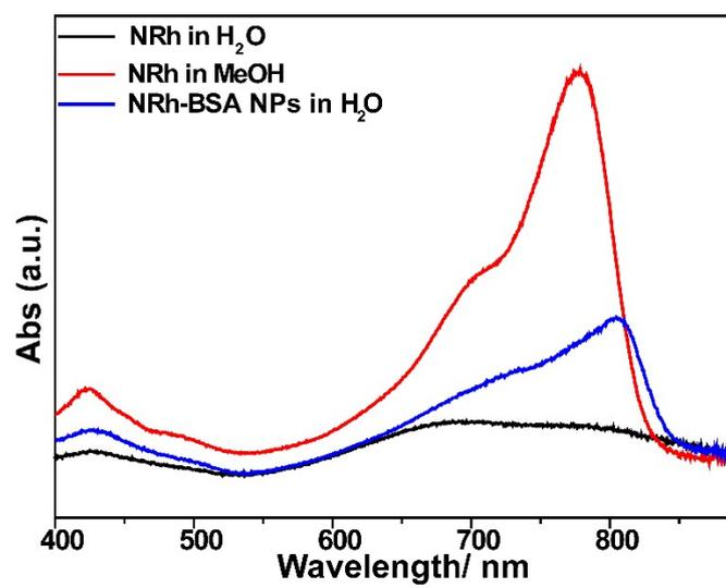
Fig. S8 Absorption spectra of NRh, NRh-BSA NPs in H<sub>2</sub>O and NRh in MeOH.
