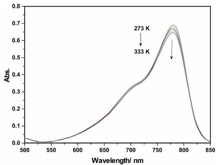
**Fig. S4** Absorption spectra NRh in ethanol at different temperatures.
