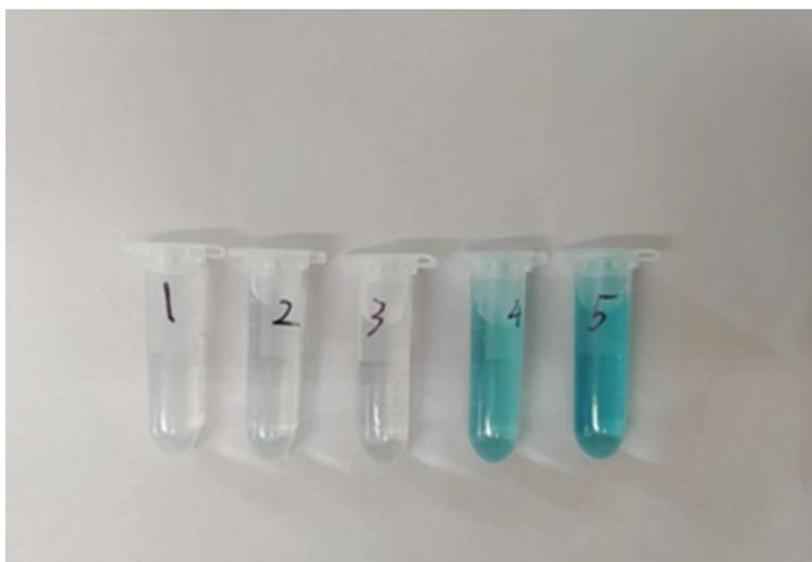
**Figure S6.** The photograph of TMB solution color change. (1) TMB; (2) TMB+H<sub>2</sub>O<sub>2</sub>; (3) TMB+H<sub>2</sub>O<sub>2</sub>+AIO; (4) TMB+H<sub>2</sub>O<sub>2</sub>+AIO+EDTA; (5) TMB+H<sub>2</sub>O<sub>2</sub>+AIO-EDTA.
