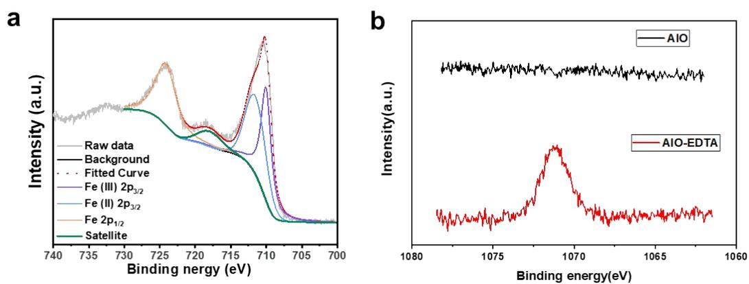
**Figure S3.** (a) X-ray photoelectron spectroscopy (XPS) high-resolution scans of Fe 2p peaks in AIO NPs. (b) XPS high-resolution scans of Na 1s peaks in AIO NPs and AIO-EDTA NPs. Compared with AIO NPs, the appearance of Na 1s peaks in AIO-EDTA NPs suggests EDTA is successfully loaded into AIO NPs.
