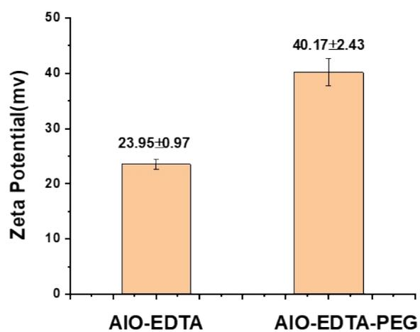
**Figure S4.** Zeta potentials of AIO-EDTA NPs with or without PEG modifications detected by dynamic light scattering.
