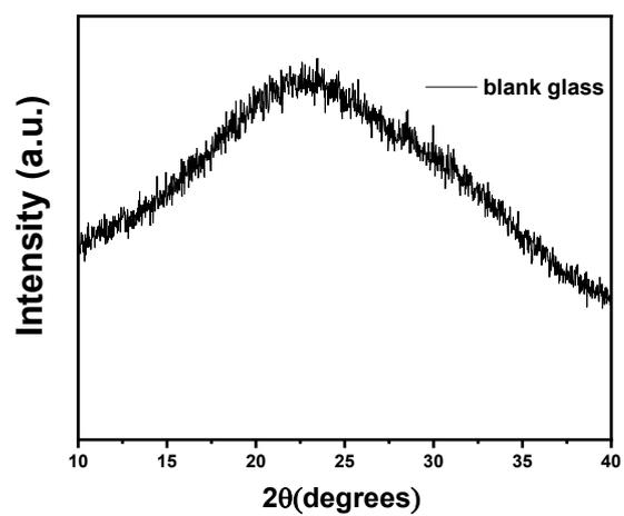
**Figure S2.** PXRD pattern of blank glass sheet.
