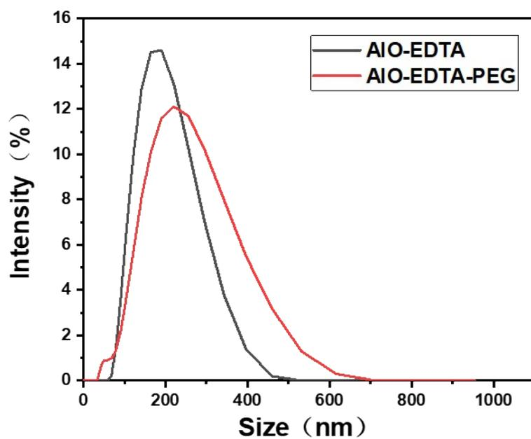
**Figure S1.** The hydrodynamic sizes of AIO-EDTA NPs and AIO-EDTA-PEG NPs in H<sub>2</sub>O detected by dynamic light scattering.
