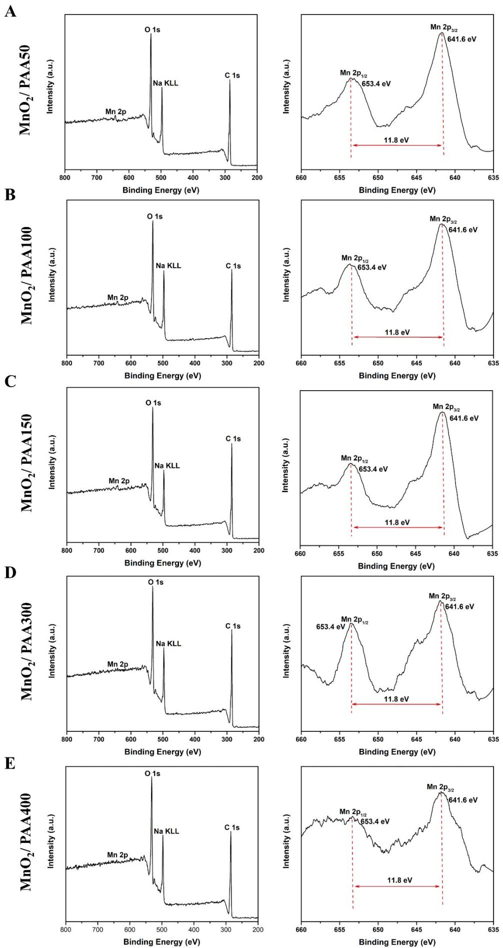
Figure S1. XPS spectra of MnO<sub>2</sub>/PAA50 NPs and Mn 2p (A), MnO<sub>2</sub>/PAA100 NPs and Mn 2p (B), MnO<sub>2</sub>/PAA150 NPs and Mn 2p (C), MnO<sub>2</sub>/PAA300 NPs and Mn 2p (D), MnO<sub>2</sub>/PAA400 NPs and Mn 2p (E).
