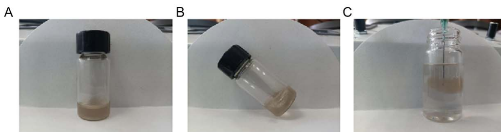
Figure S5. The gel phenomenon of nanoparticles in calcium ion environment. A) GdOF @ PDA-HA-R837 HG was mixed with \text{Ca}^{2+} solution. B) The mixed solution of A) was tilted and shown a gel formation rather than a liquid. C) GdOF @ PDA-HA-R837 HG was added to \text{Ca}^{2+} solution, and gel formation appeared immediately.
