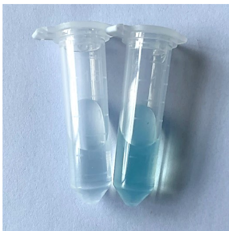
Figure S10. The photograph of TMB treated with H_2O_2 (left) and H_2O_2+PNC (right).
