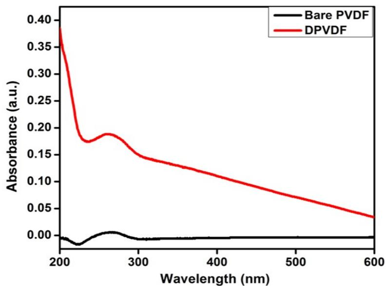
**Fig. S2:** UV-Visible absorbance spectra of DPVDF and PVDF nanospheres.
