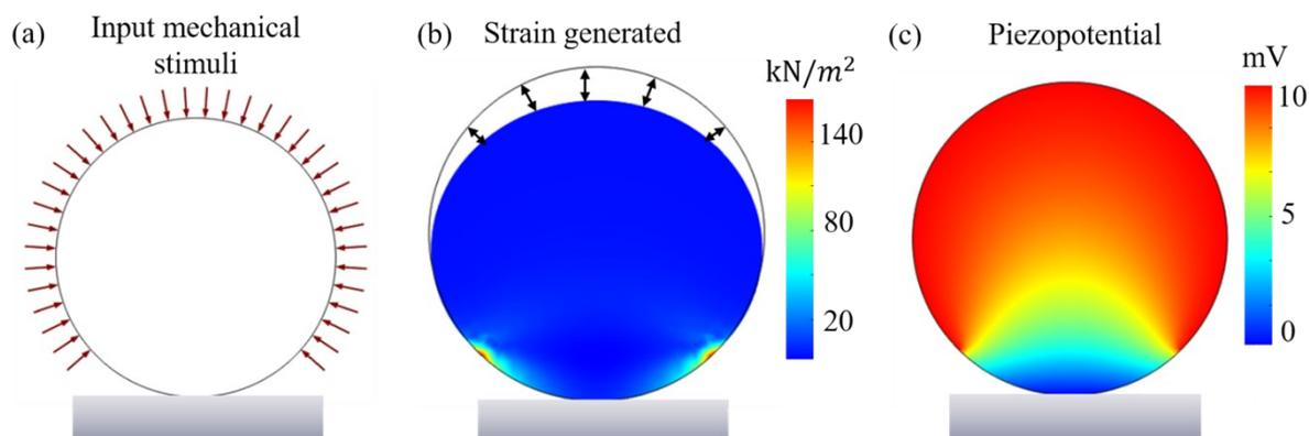
**Fig. S4.** (a) Scheme demonstrating the input mechanical stimuli (shown by arrows) of  $100 \text{ kN/m}^2$  provided to the PVDF nanosphere. (b) Strain generation within the nanosphere (as per FEA analysis) due to the input mechanical agitation (double headed arrows indicate the
