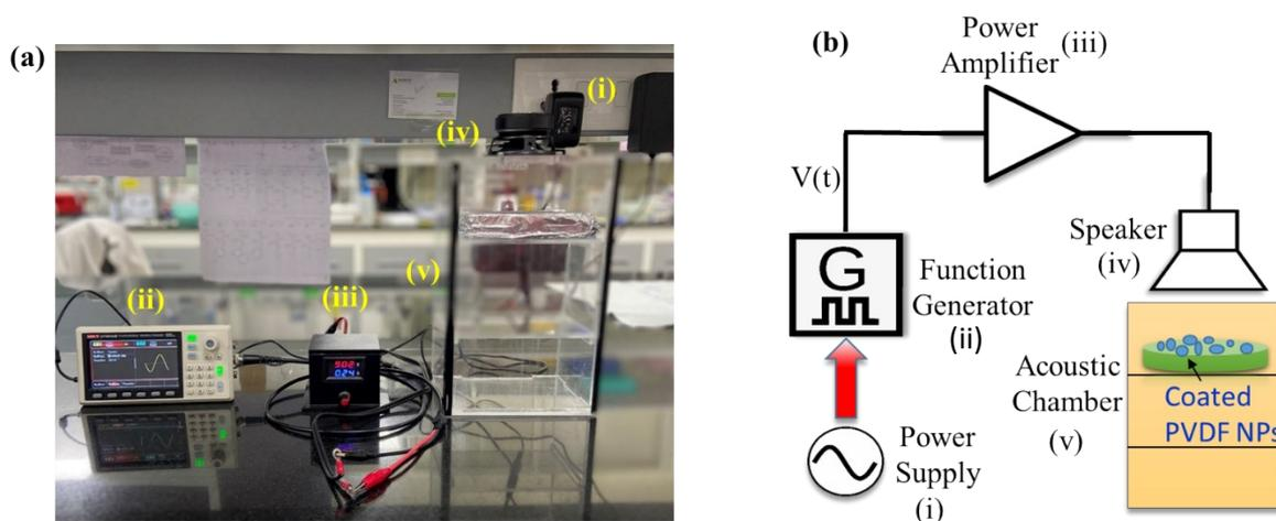
**Fig. S11.** (a) Image showing the acoustic chamber used in the study for achieving acoustic stimulation-based activation of the nanospheres. (b) Equivalent circuit diagram comprising of (i) power supply, (ii) function generator, (iii) power amplifier and (iv) speaker for the mechanical stimulation in the acoustic chamber (iv) where the ‘specimen of study’ was placed.
