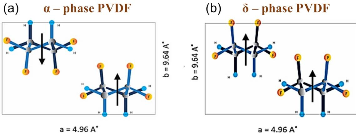
**Fig.S1:** Unit cell chemical structure of (a)  $\alpha$ -phase and (b)  $\delta$ -phase PVDF.
