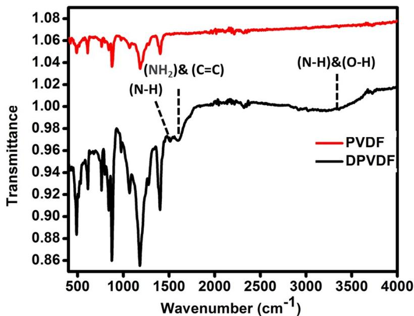
**Fig. S3:** ATR-FTIR spectra of DPVDF and PVDF nanospheres.
