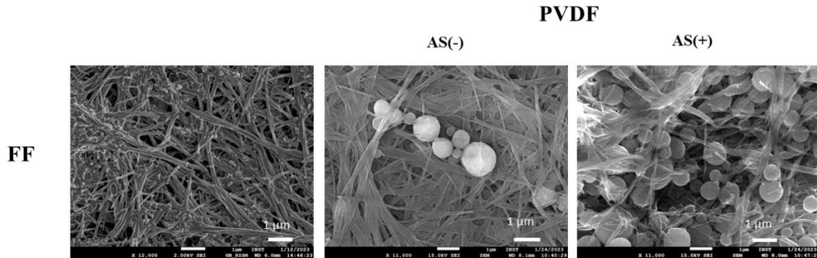
**Fig. S5:** FESEM images showing no significant structural and morphological transitions of FF fibrils after being treated with acoustic stimulus activated and non-activated PVDF nanospheres (Scale bars are 1 μm).
