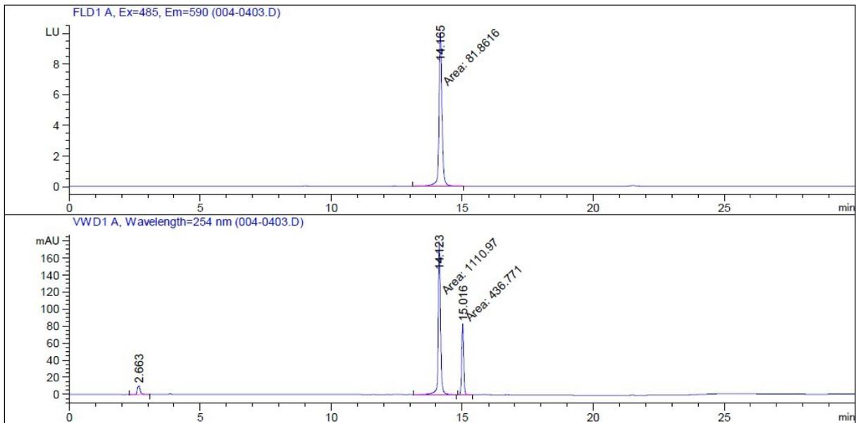
Figure S8 – Representative chromatograms for a Dox/Ola standard at 10 µg/mL. Top: FLD response at 485/590 nm (ex/em) showing Dox peak at 14.165 min. Bottom: VWD response at 254 nm showing Dox peak at 14.123 min and Ola peak at 15.016 min
