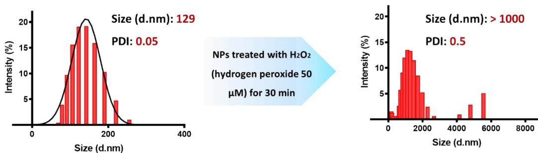
Figure S5 – Disruption of oxidation-sensitive NPs via hydrogen peroxide. Micellar-like NPs of ~ 130 nm (left) no longer form discrete stable nanoparticles resulting in the appearance of aggregates in light-scattering experiments (right).
