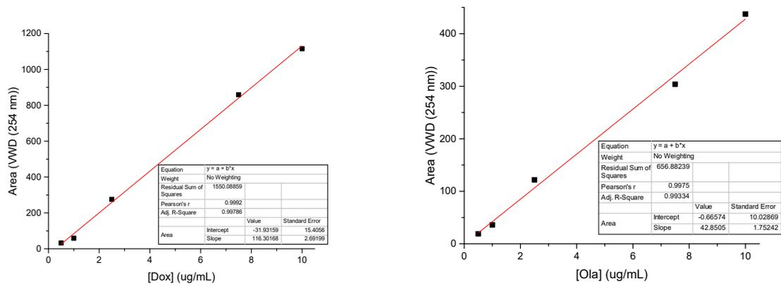
Figure S9 – Calibration curves of a) Doxorubicin and b) Olaparib using the VWD response
