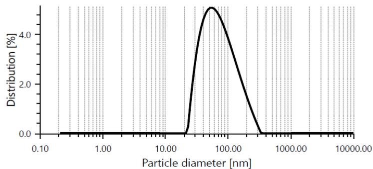
**Figure S.2.6.2:** Particle Size Distribution (Intensity) plot in Water
