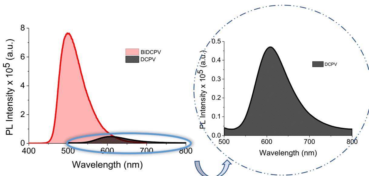
**Figure S.2.1.1:** Solid State Fluorescence comparison of DCPV and BIDCPV.
