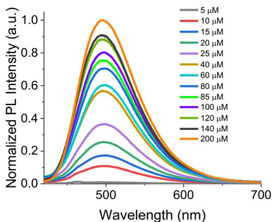
Figure S.2.8.1: Normalized PL. spectra of BIDCPV in water having different concentration
