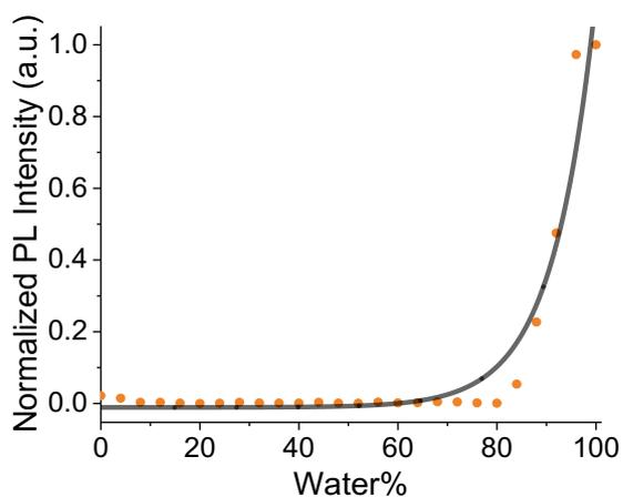
Figure S.2.2.4: Relative increase in Fluorescence due to Aggregation
