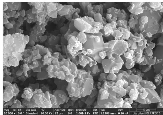
**Figure S.2.5.10: Powdered by 20 mins grinding**
