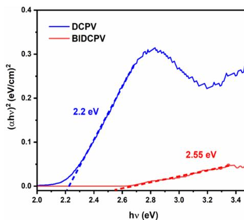
Figure S.2.7.3: In Solid state HOMO-LUMO energy gap of DCPV (blue) and BIDCPV (red) from DRS data.
