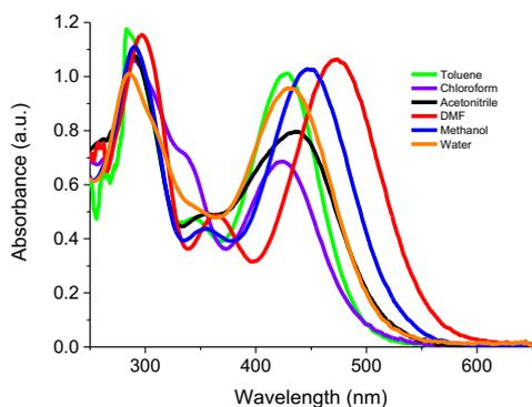
**Figure S.2.11.1:** UV-Vis Absorbance spectra of DCPV in different solvents
