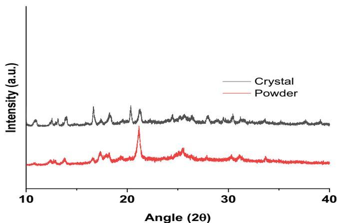
Figure S.2.4.1: PXRD data of Crystal and powdered samples of DCPV
