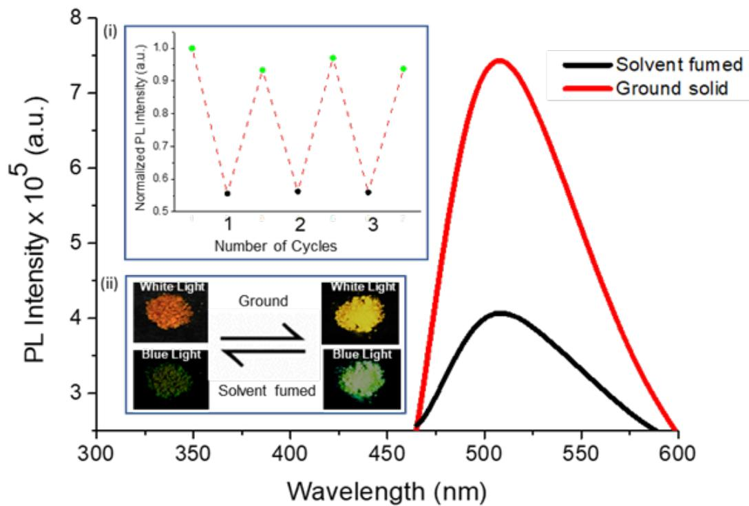
**Figure S.2.1.3:** Comparison of solid state fluorescence of BIDCPV in solvent fumed crystalline and ground form. Inset – (i) Fluorescence switchability of BIDCPV by solvent fuming / ground and (ii) White and Blue light pictures of Dark and Bright fluorescence states of BIDCPV tuned by Solvent Vapour.
