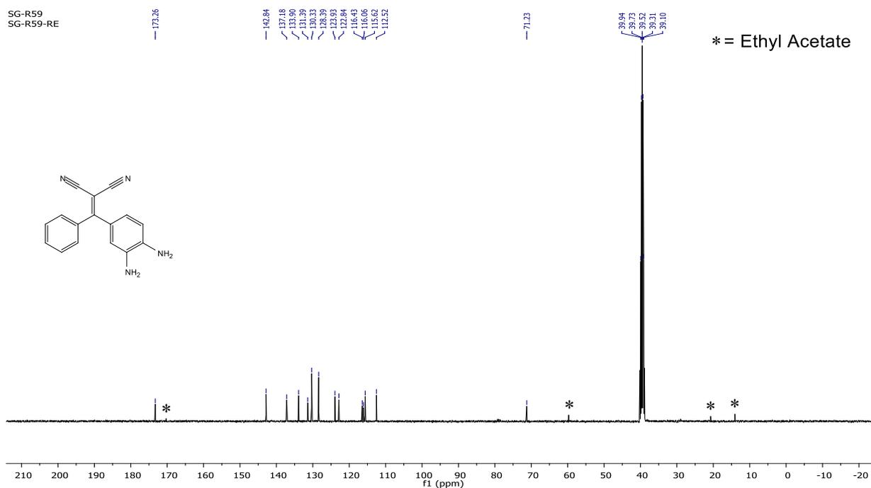
Figure S.4.1.2:  $^{13}\text{C}$  NMR data of DCPV
