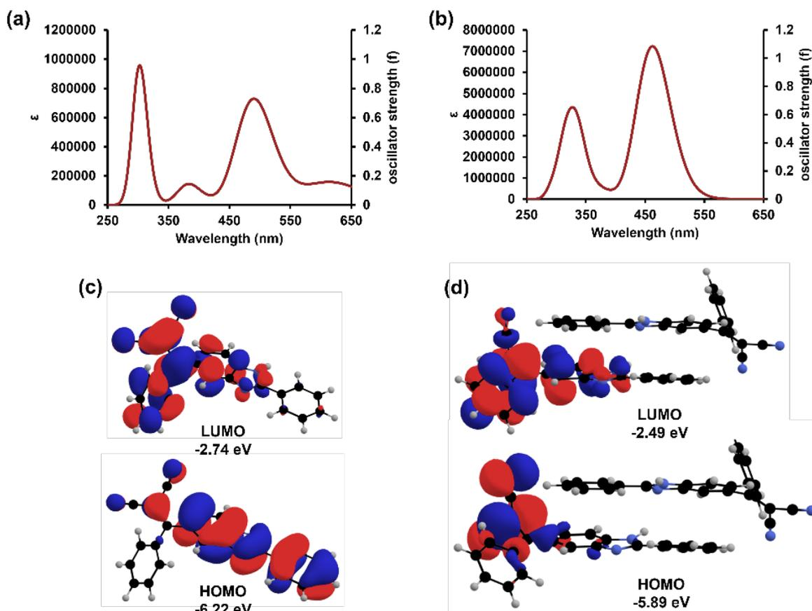
**Figure S.5.3:** TD-DFT calculated emission spectrum for BIDCPV (a) monomer, (b) dimer and their corresponding frontier molecular orbital for (c) monomer and (d) dimer the ground singlet  $S_0$  state. Notably, as expected the HOMO-LUMO energy gap reduces by 0.08 eV in the optimized dimer of BIDCPV.
