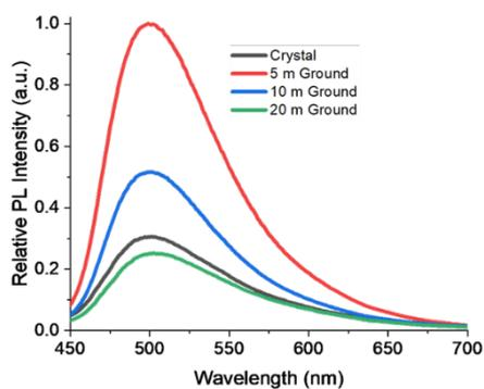
**Figure S.2.12.1:** Fluorescence Emission spectra of different states of BIDCPV during grinding.
