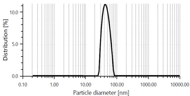
**Figure S.2.6.1:** Particle Size Distribution (Intensity) plot in Chloroform
