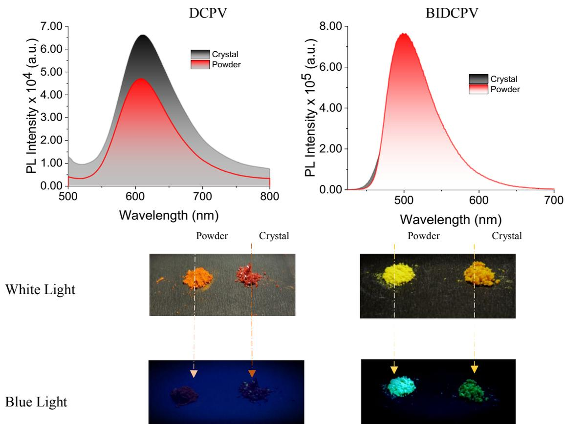
**Figure S.2.1.2:** Crystal and Powder form Solid State Fluorescence comparison of DCPV and BIDCPV.
