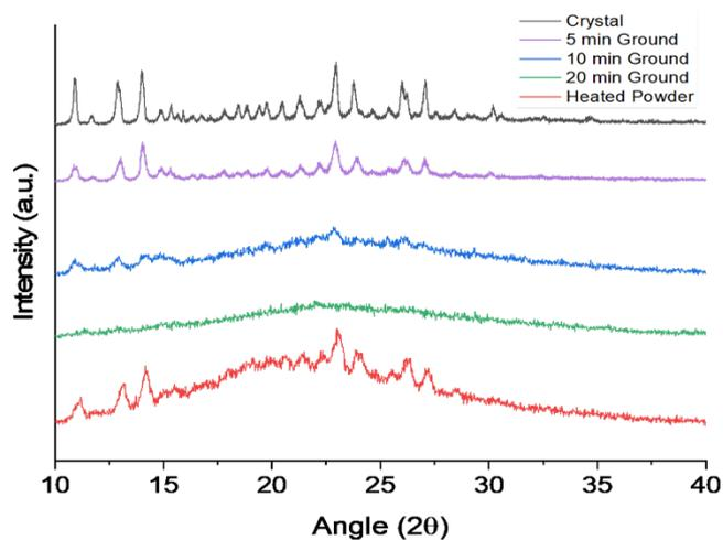
Figure S.2.4.2: PXRD data for confirmation of heat reversibility of crystallinity for BIDCPV
