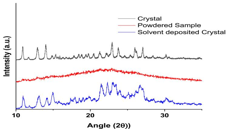
Figure S.2.4.3: PXRD data of BIDCPV for confirmation of reversibility of crystallinity by DCM vapour deposition
