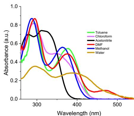
**Figure S.2.11.2:** UV-Vis Absorbance spectra of BIDCPV in different solvents
