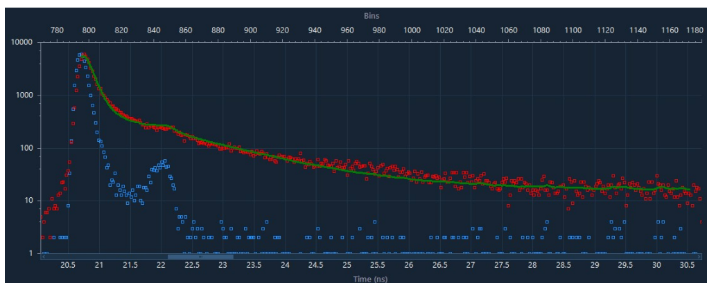
Figure S12. TRPL of 2 before photoreaction (blue dots: instrument response function; red dots: sample measurement).
