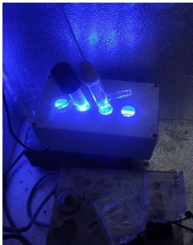
**Figure S1.** Photoreactor used in this study in a refrigerator to keep the temperature at 10 °C
