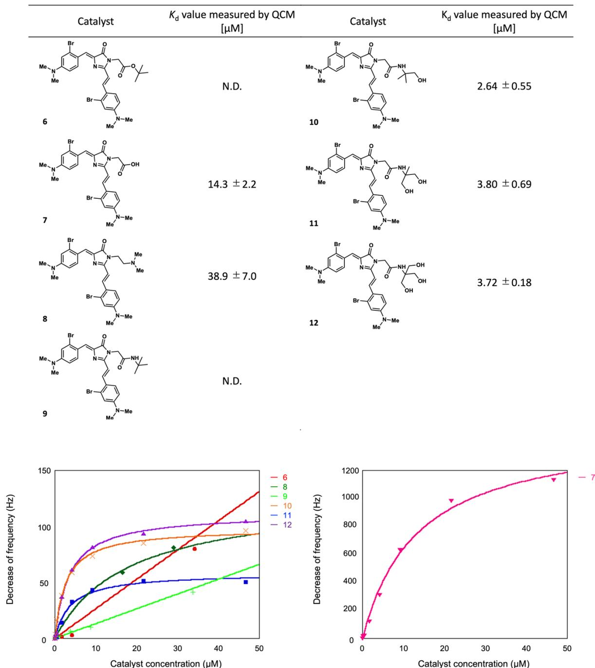
The  $K_d$  value of catalyst **6** and **9** was not obtained under the identical conditions (= N.D.). The low water solubility may have caused the catalyst to bind the sensor nonspecifically, resulting in a linear plot.
