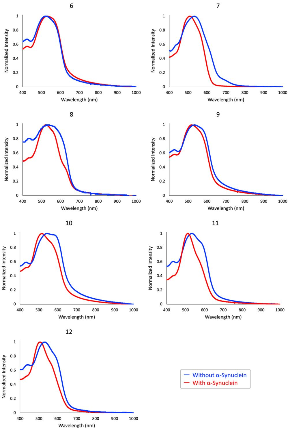
A phosphate buffer solution (pH 7.4) containing catalyst (20  $\mu$ M) in the presence or absence of aggregated  $\alpha$ -synuclein (20  $\mu$ M) was incubated at 37  $^{\circ}$ C for 10 min and absorbance spectra were measured.
