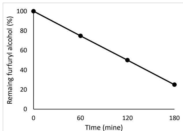
Glycerol/methanol = 1/1 solvent containing **11** (20  $\mu\text{M}$ ) and furfuryl alcohol (FurA; 2 mM) was photo-irradiated ( $\lambda = 500 \text{ nm}$ ) at room temperature for certain time periods, and the remaining FurA was quantified by ultraviolet (UV) absorbance.
