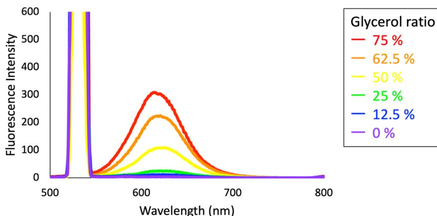
To each ratio of glycerol-PBS mixed solvents (glycerol: 0, 12.5, 25, 50, 62.5, and 75 %) catalyst **11** was added at the final concentration of 2  $\mu$ M, and the fluorescence spectra were measured.
