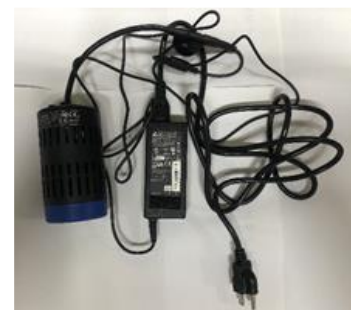
Kessil PR160L-456 nm blue LED light and supporting power cables outside the box
