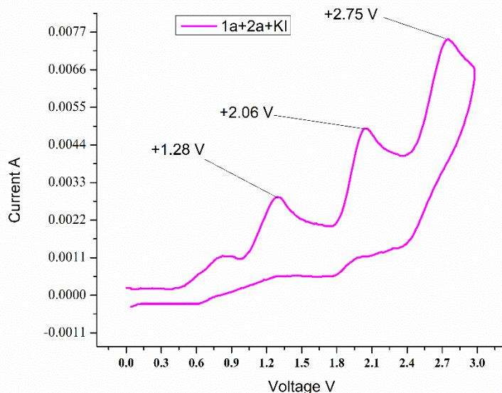
**Figure S4.** Cyclic voltammograms of reactants and mixture in 0.1 M *n*-Bu<sub>4</sub>NPF<sub>6</sub>/ CH<sub>3</sub>CN (3:2)
