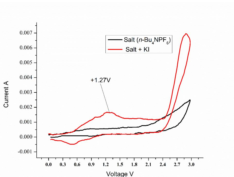
**Figure S1.** Cyclic voltammograms of reactants and mixture in 0.1 M *n*-Bu<sub>4</sub>NPF<sub>6</sub>/ CH<sub>3</sub>CN (3:2) using a glassy carbon disk electrode, Pt electrode as counter electrode and Ag/AgCl as reference
