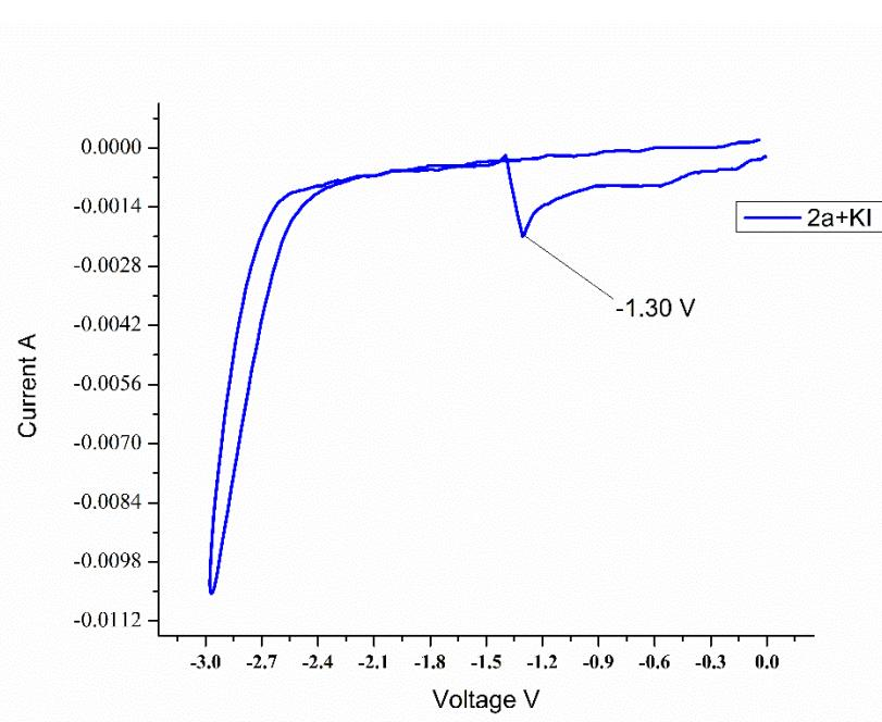
**Figure S2.** Cyclic voltammograms of reactants and mixture in 0.1 M *n*-Bu<sub>4</sub>NPF<sub>6</sub>/ CH<sub>3</sub>CN using
