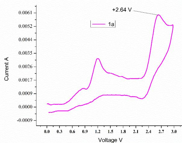
**Figure S3.** Cyclic voltammograms of reactants and mixture in 0.1 M *n*-Bu<sub>4</sub>NPF<sub>6</sub>/ CH<sub>3</sub>CN using a glassy carbon disk electrode, Pt electrode as counter electrode and Ag/AgCl as reference electrode, at a 200 mVS<sup>-1</sup> (Curve 1a): **1a** (5 mM) + *n*-Bu<sub>4</sub>NPF<sub>6</sub> (0.05 M), KI (0.025M)
