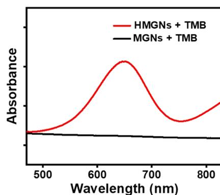
Figure S13. The UV-Vis absorbance spectra of TMB treated by MGNs and HMGNs in a pH 4.0 phosphate solution.
