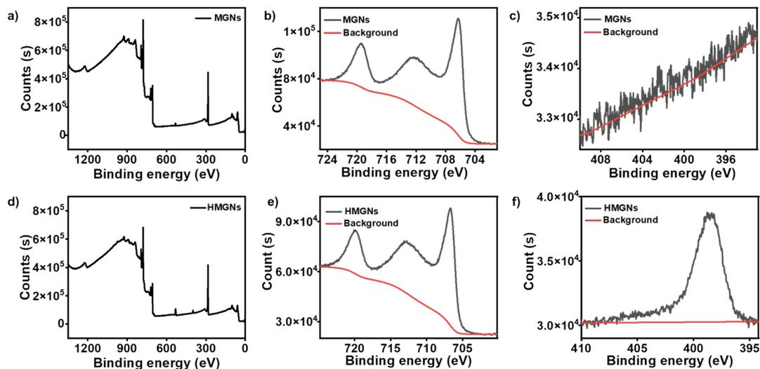
Figure S10. (a) XPS survey spectra of MGNs. High-resolution XPS spectra of (b) Fe 2p<sub>3</sub> and (c) N 1s for MGNs. (d) XPS survey spectra of HMGNs. High-resolution XPS spectra of (e) Fe 2p<sub>3</sub> and (f) N 1s for HMGNs.
