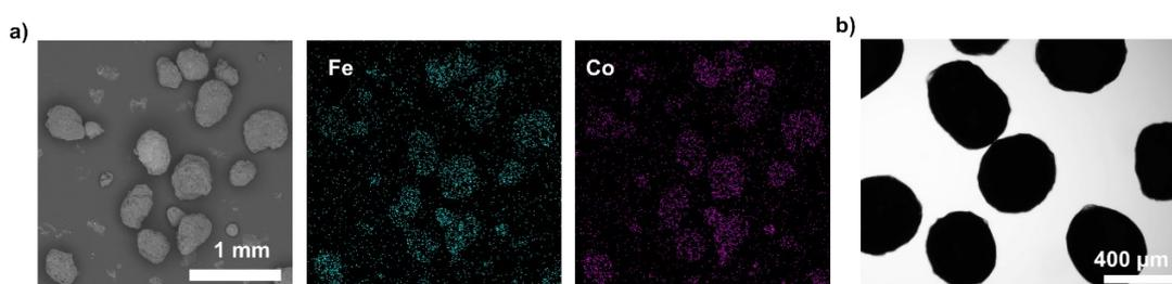
Figure S3. Characterization of FCSMGs. (a) SEM image and corresponding EDS mapping of FCSMGs. (b) Microscopy imaging of FCSMGs.
