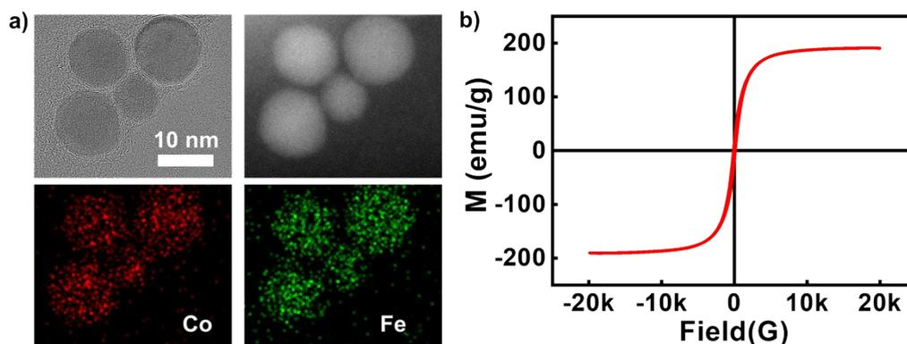
Figure S2. Characterization of MGNs. (a) TEM image and corresponding EDS mapping of MGNs. (b) Field-dependent magnetization hysteresis loop of the MGNs at room temperature.
