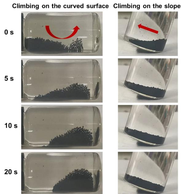
Figure S6. The climbing motion of the micro-sweepers on the curved surface and the sloping underside of the glass bottle.
