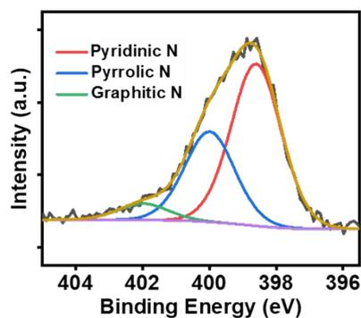
Figure S11. High-resolution XPS spectra of N 1s for HMGNs.
