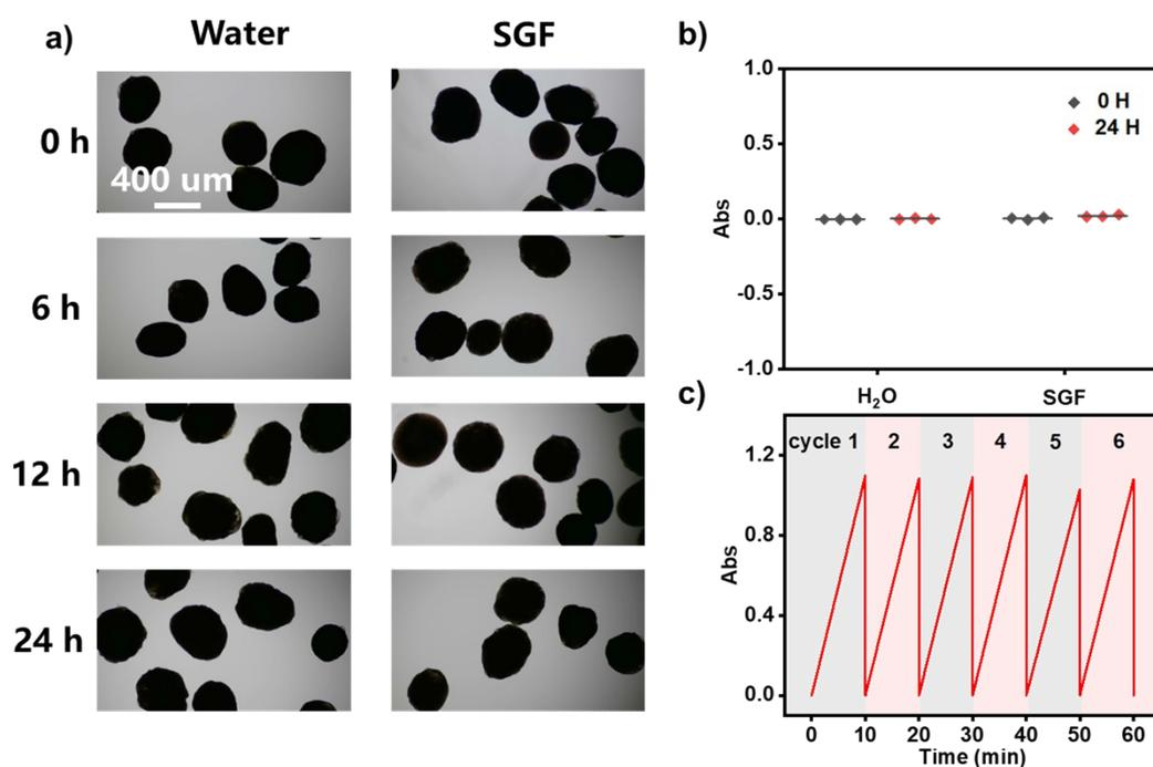
Figure S14. (a) Microscopy images of FCSHMGNs during 24-hour incubation with water and SGF. (b) The UV-Vis absorbance at 280 nm of the 24-hour supernatant from Figure S14a. (c) The catalytic ability of FCSHMGNs in six cycles.
