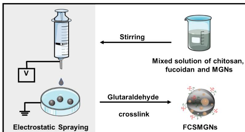
Figure S1. The scheme of FCSMGs preparation using electrostatic spraying method. Briefly, the mixture of fucoidan, chitosan and magnetic graphitic MGNs was electrostatically sprayed in a 10 kV-electrostatic field and cross-linked by glutaraldehyde to obtain FCSMGs.
