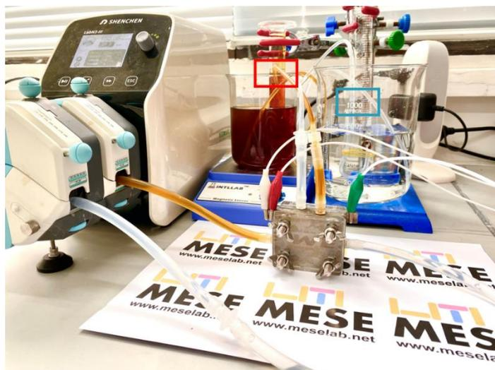
**Fig. S14** Digital photograph of the set-up of the acid/alkaline furfural hybrid battery to measure  $H_2$  Faradaic efficiency at both the cathode and anode.
