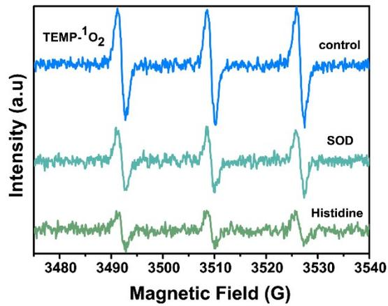
**Fig. S8** The ESR spectra of <sup>1</sup>O<sub>2</sub> with adding SOD and HIS.
