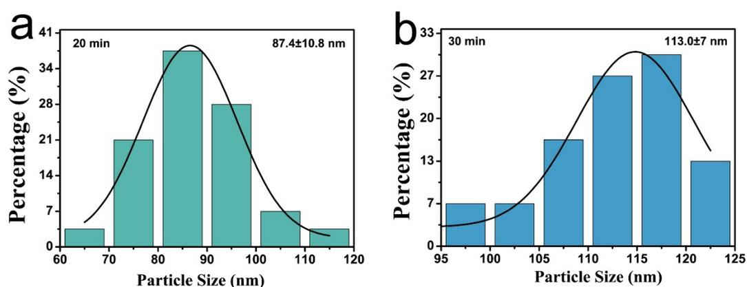
**Fig. S10** Particle size of ZrTCPP at different reaction time.
