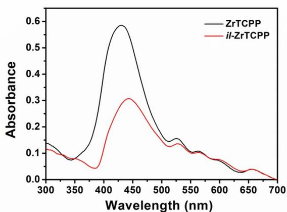
**Fig. S4** UV-vis spectrum of ZrTCPP (black line) and *il*-ZrTCPP (red line).
