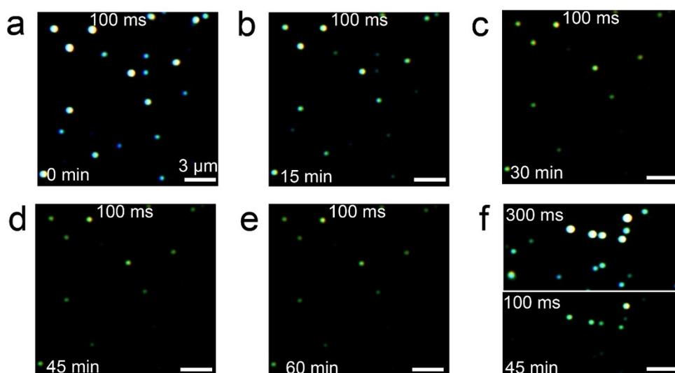
**Fig. S2** DFM images of nano-sized ZrTCPP at different illumination time with different exposure time. (a)-(e) Dynamic DFM images of nanosized ZrTCPP particles in ultrapure water for 60 min continuous illumination with the exposure time of 100 ms. (f) DFM images for 45 min illumination with the exposure time of 100 ms and 300 ms, respectively.
