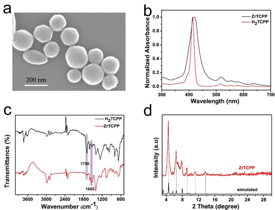
**Fig. S1** Characterization of synthesized ZrTCPP. SEM image (a), UV-vis adsorption spectrum (b), FTIR-spectra (c) and XRD spectra of ZrTCPP (d).
