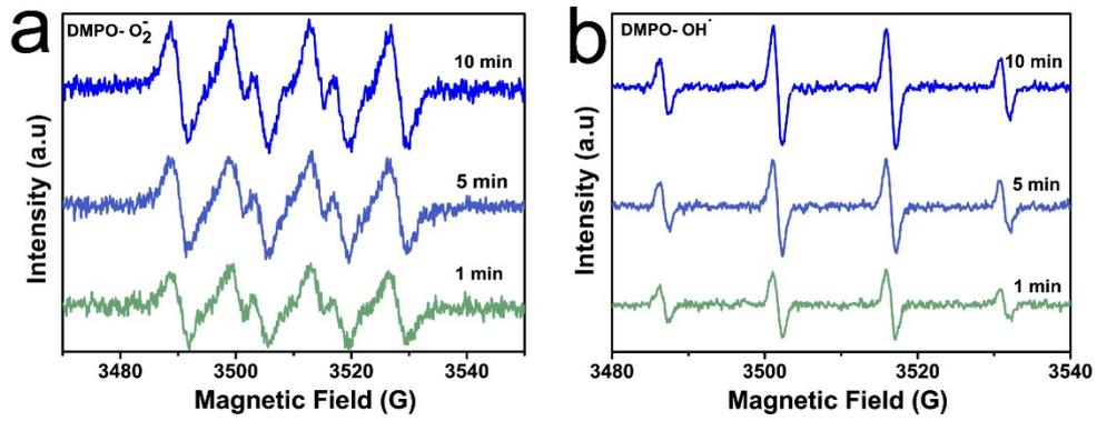
**Fig. S7** The ESR spectra of DMPO-O<sub>2</sub><sup>-</sup> (a) and DMPO-OH<sup>•</sup> (b) in the ZrTCPP-H<sub>2</sub>O system under illumination.
