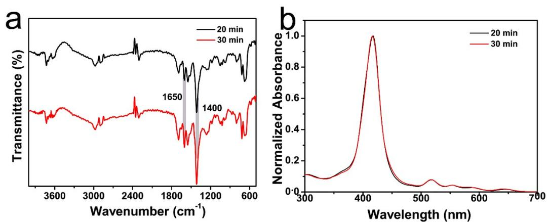
**Fig. S11** FTIR-spectra (a) and UV-spectra (b) characterization of ZrTCPP at 20 min (black line) and 30 min (red line).
