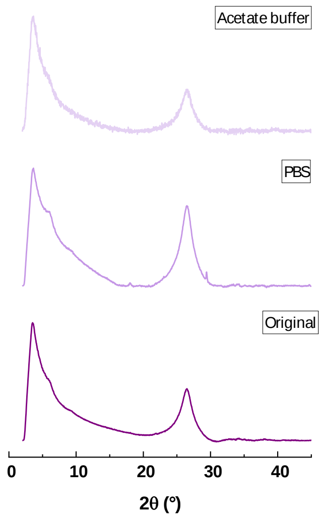
Figure S15. PXRD pattern of NI-COF following the stability tests in PBS and acetate buffers.
