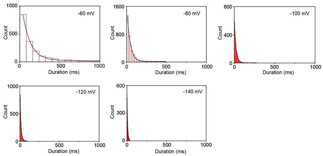
Fig. S7 The histograms of inter-event intervals for  $\beta$ -CD in Aep1 nanopore at different voltages.
