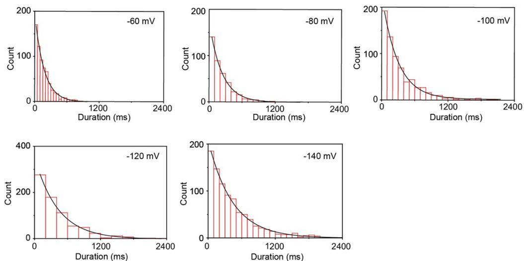
Fig. S10 The duration histograms of  $\gamma$ -CD in Aep1 nanopore at different voltages.
