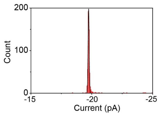
Fig. S12 The histogram of blockage current of  $\gamma$ -CD in Aep1 nanopore at -140 mV.
