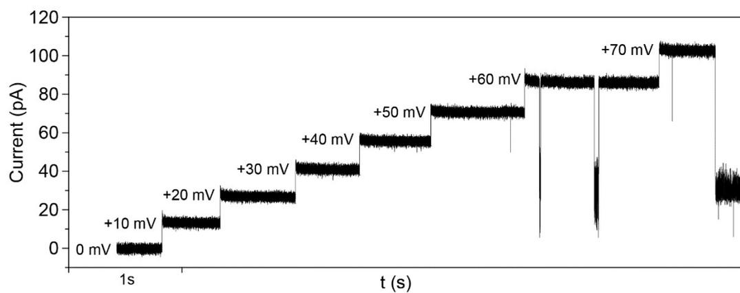
Fig. S1 The voltage-dependent gating events in Aep1 nanopore at pH 8.0/8.0 (*cis/trans*).
