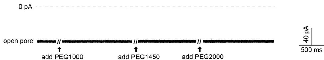
Fig. S11 The ionic current trace in Aep1 nanopore after the successive addition of PEG1000, PEG1450 and PEG2000 both into *cis* and *trans* side at - 80 mV.
