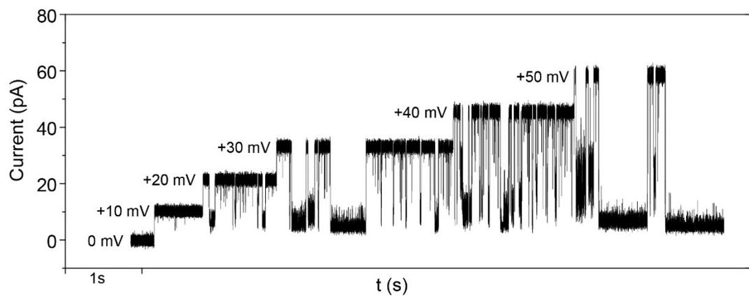
Fig. S2 The voltage-dependent gating events in Aep1 nanopore at pH 5.0/5.0 (*cis/trans*).
