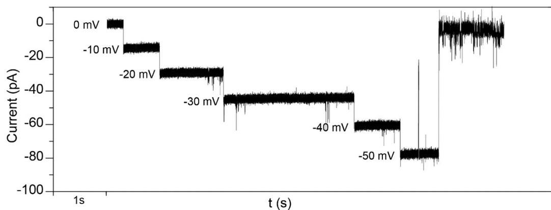
Fig. S3 The voltage-dependent gating events in Aep1 nanopore at pH 8.0/5.0 (*cis/trans*).
