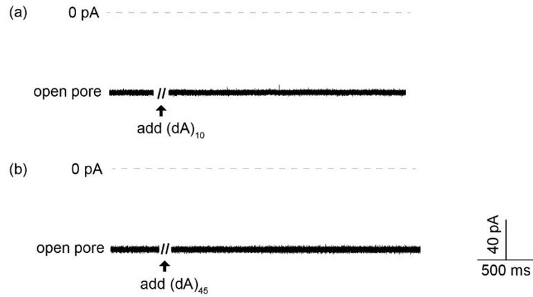
Fig. S4 The ionic current traces in Aep1 nanopore after the addition of (dA)<sub>10</sub> (a) or (dA)<sub>45</sub> (b) both into *cis* and *trans* side at - 80 mV.
