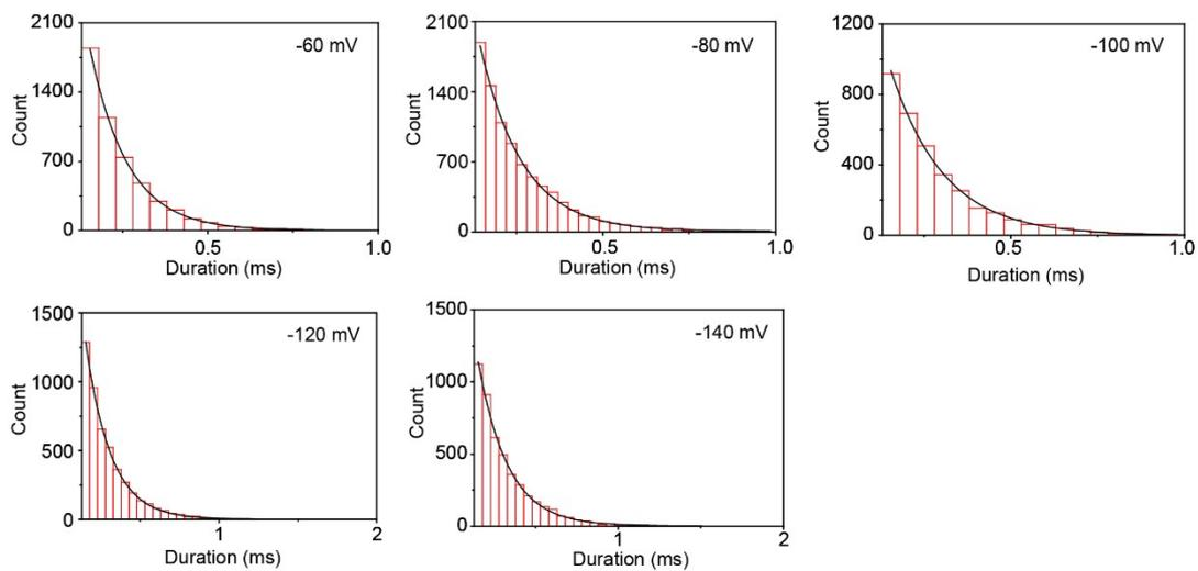
Fig. S9 The duration histograms of  $\beta$ -CD in Aep1 nanopore at different voltages.
