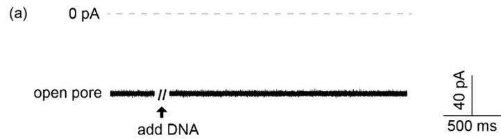
Fig. S5 The ionic current trace in Aep1 nanopore after the addition of DNA with a hairpin structure both into *cis* and *trans* side at - 80 mV.
