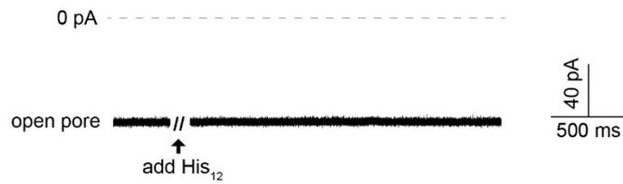
Fig. S6 The ionic current trace in Aep1 nanopore after the addition of His<sub>12</sub> both into *cis* and *trans* side at - 80 mV.
