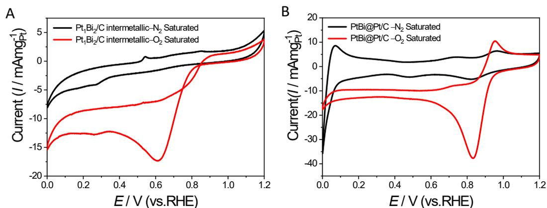
Figure S8. CV curves of (A) the Pt<sub>1</sub>Bi<sub>2</sub>/C intermetallic and (B) PtBi@Pt/C in an aqueous solution of KOH (0.1 M) at room temperature recorded at a scan rate of 50 mV s<sup>-1</sup>. The current densities were normalized against the mass of Pt loaded on the electrodes.
