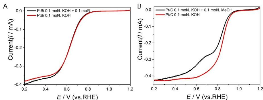
Figure S9. Polarization curves for the ORR. (A) PtBi@Pt/XC-72 catalyst; (B) Pt/C NPs. Conditions: in O<sub>2</sub>-saturated 0.1 mol/L KOH that contained 0 and 0.1 mol/L methanol at a rotation rate of 900 rpm. Sweep rate: 10 mV/s.
