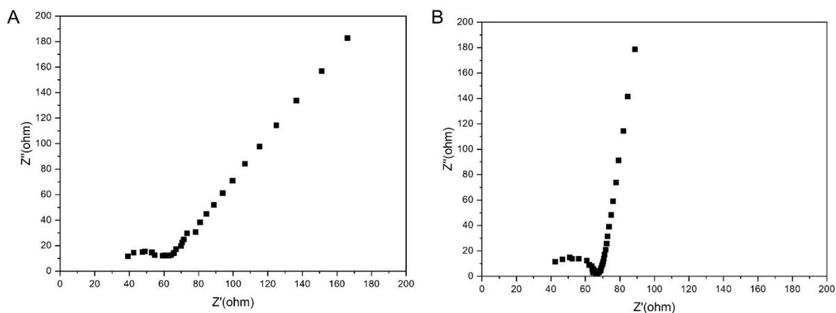
Figure S11. Nyquist plots of the corresponding catalysts of PtBi@Pt/C (A) and Pt/C (B).
