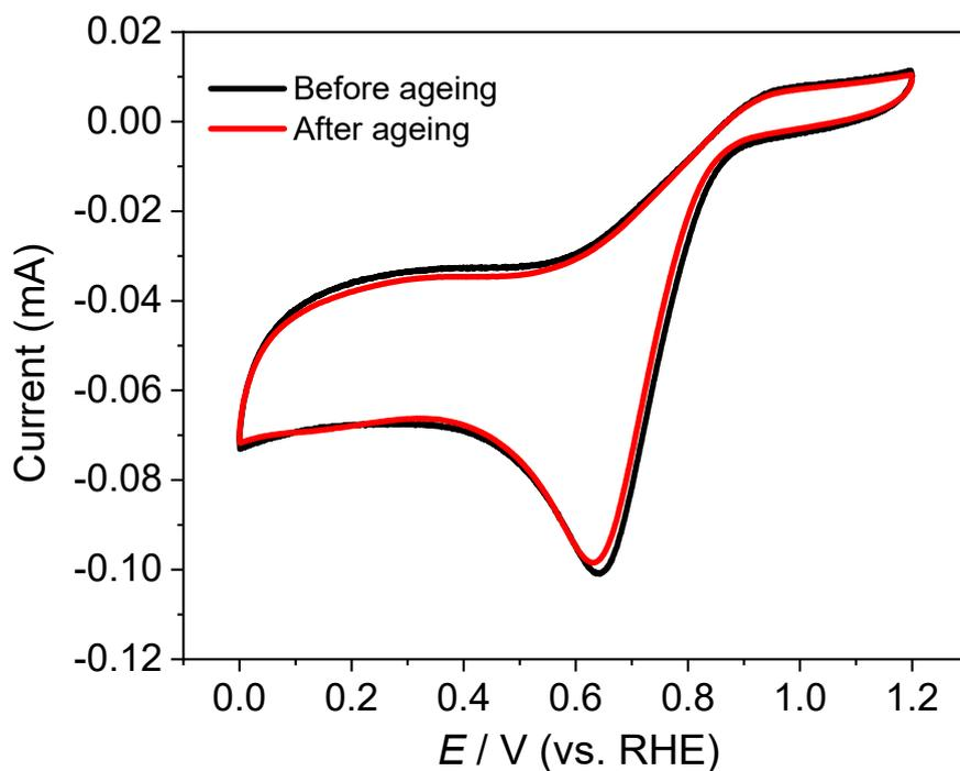
Figure S10. Stability test for PtBi@Pt/C. Before and after aging for 1000 cycles in O<sub>2</sub>-saturated 0.1 mol/L KOH that contained 0 and 0.1 mol/L methanol. Sweep rate: 50 mV/s.
