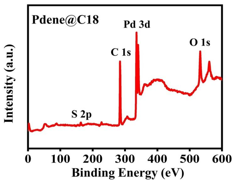
Fig. S4 XPS survey spectrum of Pdene@C18.
