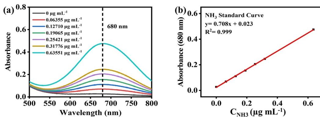
**Fig. S7** (a) The UV-vis spectra of various  $\text{NH}_4^+$  concentrations with the color reagent at room temperature for 1 h. (b) Calibration curve used for calculation of  $\text{NH}_3$  concentration.
