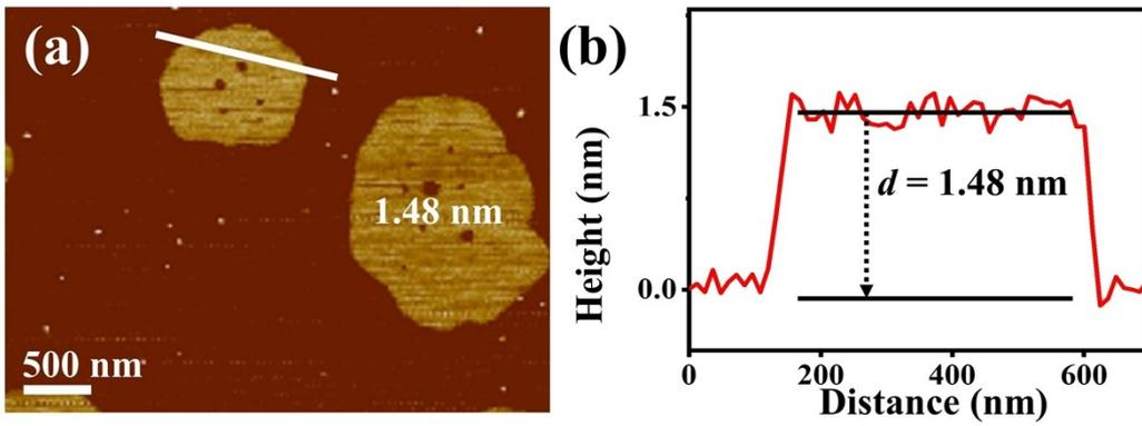
**Fig. S2** (a) AFM image and (b) corresponding height profile of Pdene.
