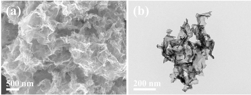
**Fig. S1** (a) SEM and (b) TEM images of Pdene.
