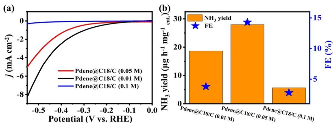
**Fig. S9** (a) LSV curves of Pdene modified with different concentrations of octadecanethiol in N<sub>2</sub>-saturated 0.1 M Na<sub>2</sub>SO<sub>4</sub> with a scan rate of 10 mV s<sup>-1</sup>. (b) Corresponding NH<sub>3</sub> yields and FEs of Pdene modified with different concentrations of octadecanethiol.
