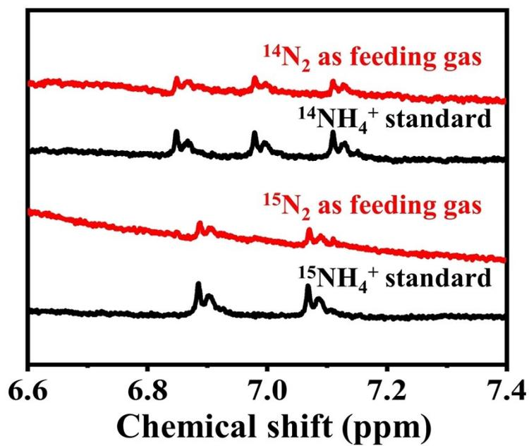
**Fig. S13**  $^1\text{H-NMR}$  spectra of both  $^{15}\text{NH}_4^+$  and  $^{14}\text{NH}_4^+$  produced from NRR process using  $^{15}\text{N}_2$  and  $^{14}\text{N}_2$  as the feeding gas, respectively.
