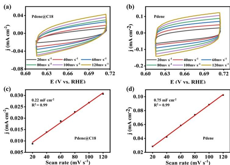
**Fig. S11** Double layer capacitance measurements at various scan rate ranging from 20-120  $\text{mV s}^{-1}$  (a) Pdene@C18 and (b) Pdene. The capacitive current densities at 0.665 V vs. RHE as a function of scan rates for (c) Pdene@C18 and (d) Pdene.
