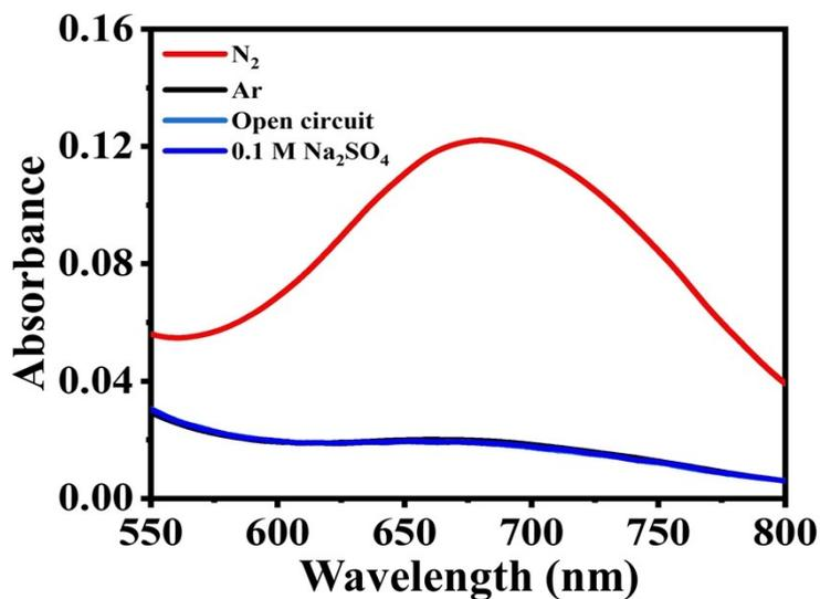
**Fig. S12** UV-vis absorption spectra of electrolysis solutions for 2 h under different conditions.
