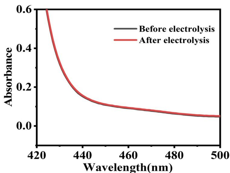
**Fig. S10** UV-vis absorption spectra of the electrolytes stained with C<sub>9</sub>H<sub>11</sub>NO indicator before and after NRR electrolysis.
