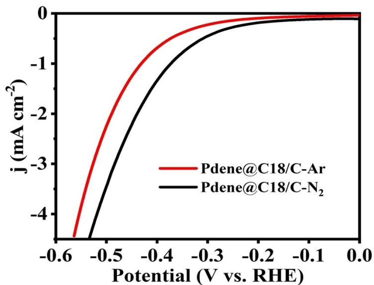
**Fig. S6** LSV curves of Pdene@C18/C in Ar- and N<sub>2</sub>-saturated 0.1 M Na<sub>2</sub>SO<sub>4</sub> with a scan rate of 10 mV s<sup>-1</sup>.
