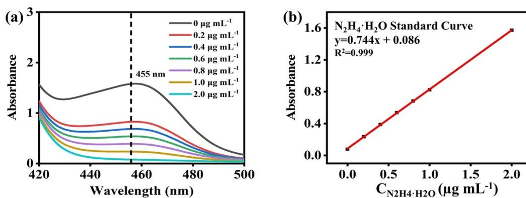
**Fig. S8** (a) UV-vis spectra of  $\text{N}_2\text{H}_4 \cdot \text{H}_2\text{O}$  with different concentrations incubated at room temperature for 15 min. (b) Calibration curve used for calculation of  $\text{N}_2\text{H}_4$  concentrations.
