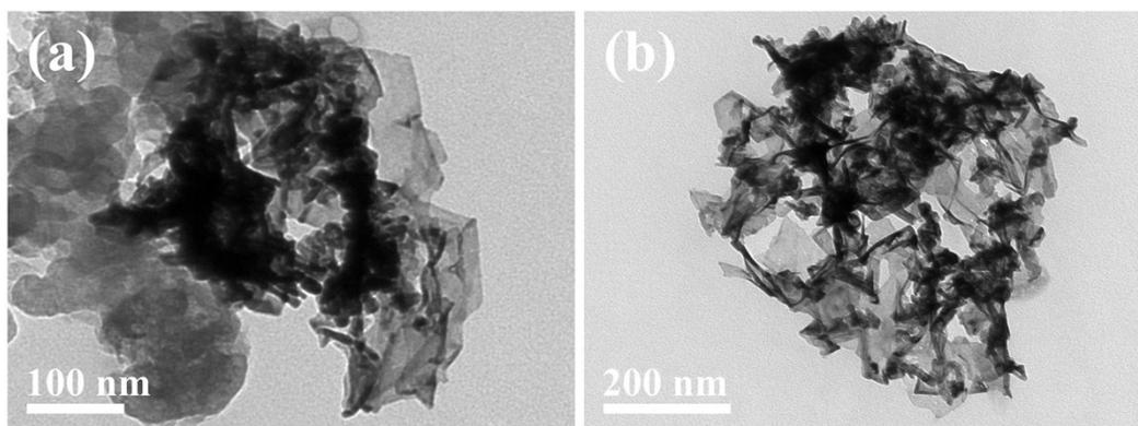
**Fig. S14** TEM images of Pdene@C18/C after stability test.
