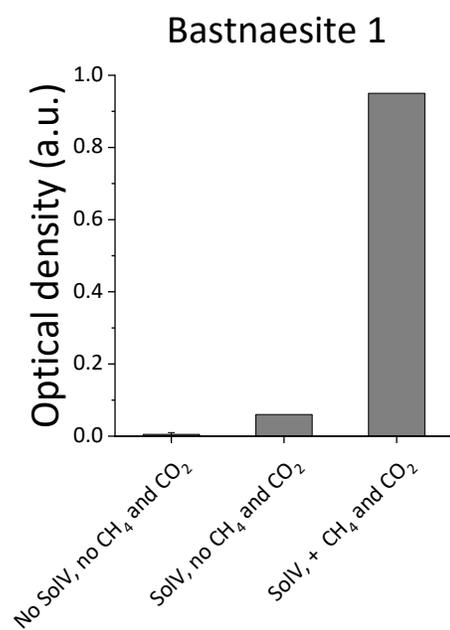
**Fig. S6.** Optical densities at 600 nm for the experiments regarding Bastnaesite 1 samples described in Fig. S3 – S5 under the different conditions. OD<sub>600</sub> was collected after 87 hours incubation at 55 °C (200 rpm).
