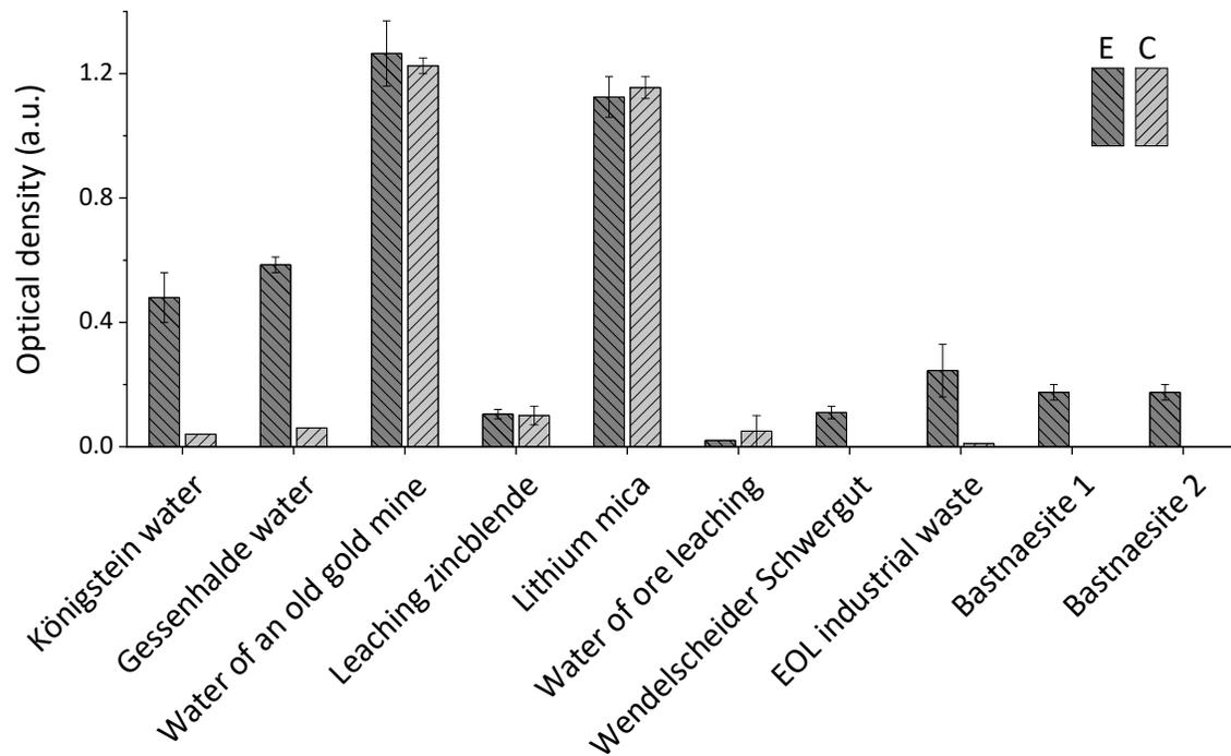
**Fig. S2.** Optical density at 600 nm for the different REE-containing sources of samples described in Fig. S1 when strain SoIV was added (E) and without added bacterial strain (C) after 3 days of cultivation. The high OD in the controls for certain sources (e.g. water of an old gold mine, Lithium mica, and leaching zinblendende) is due to precipitate formation.
