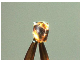
Figure S1. Selected single-crystal of investigated compound mounted on a MiTeGen micro-mount.
