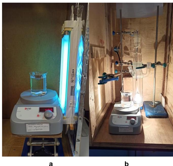
**Fig. S3.** Homogeneous oxidation system under UVA (a) and UV-Vis (or Vis) (b) used for photolytic oxidation of 3-methylpyridine.
