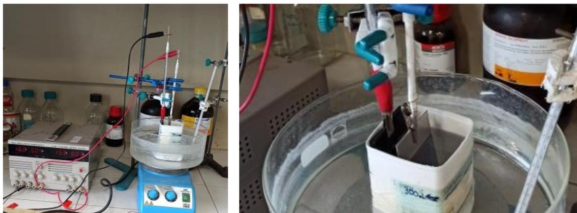
**Fig. S1.** Two-electrode system in which the anodic oxidation process is applied for nanotube-structured TiO<sub>2</sub> production on a Ti plate.
